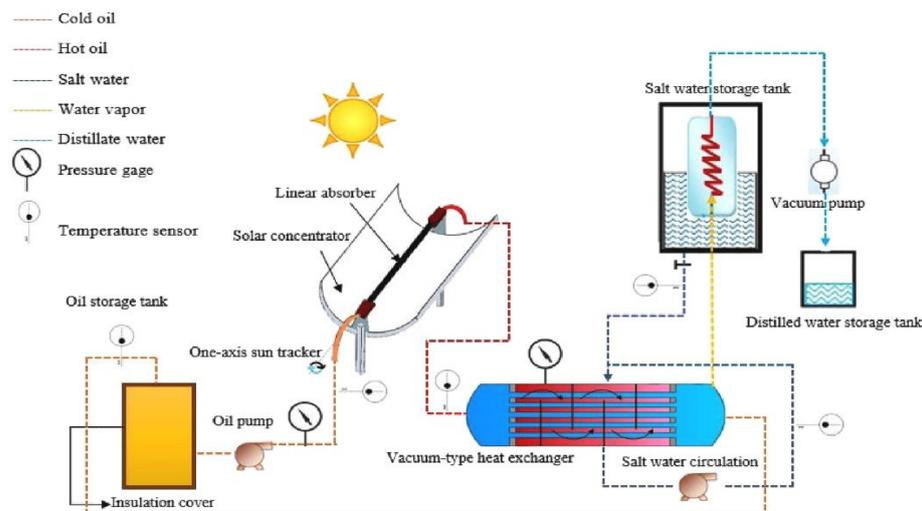
Figure 1. Schematic diagram of solar distillation system integrated with PTC and vacuum-type HE [55].
