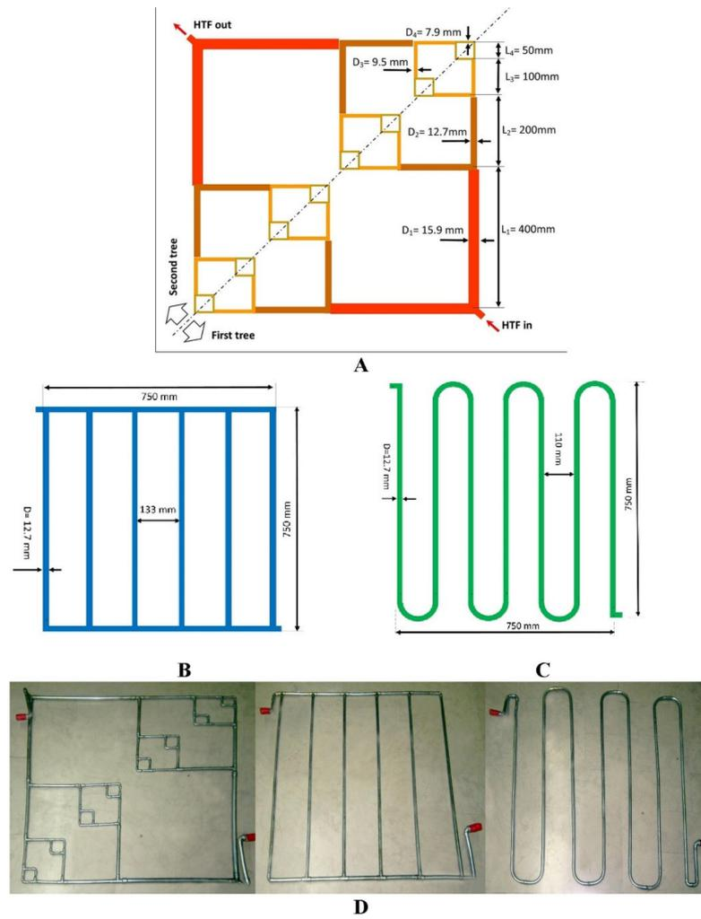
Figure 5. Different designs of heat exchangers: (A) novel design; (B) parallel channel; (C) serpentine design; (D) different designs of heat exchanger [62].
