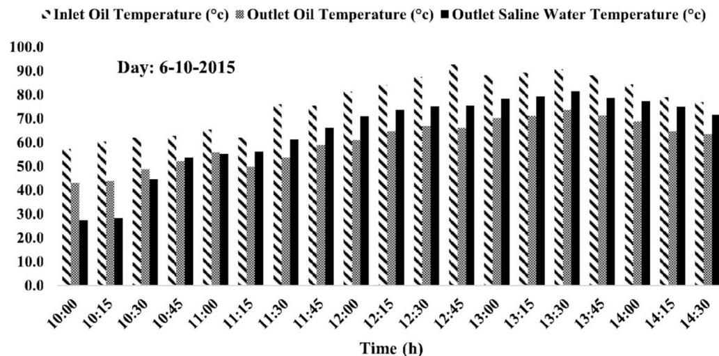
Figure 2. Differentiation in oil and water temperatures inside heat exchanger [55].
