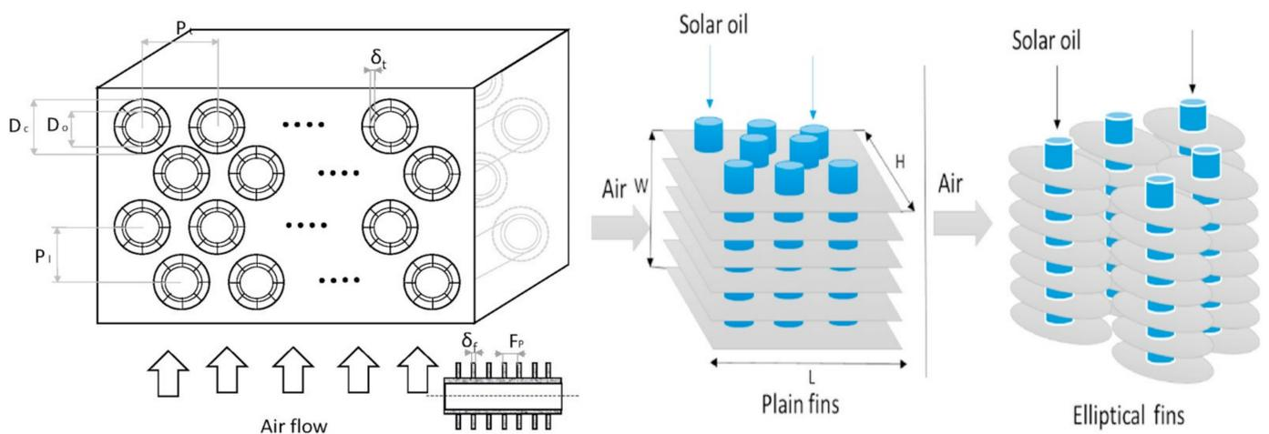
**Figure 4.** Geometry arrangement of finned tube heat exchanger [61].
