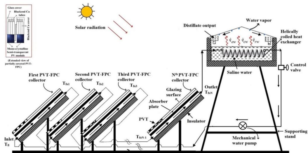
Figure 3. Schematic diagram of double-slope solar still with helical coil heat exchanger and nanofluids [57].
