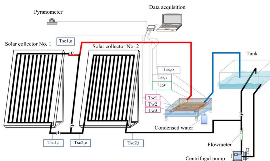
**Figure 7.** Schematic diagram of the effect of varying heat transfer coefficient of heat exchanger-equipped solar still by nanofluids [65].
