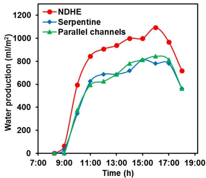
Figure 6. Hourly variation of water production for different heat exchangers [62].
