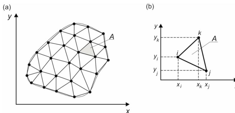
**Figure 1.** Spatial discretization: (a) domain covered by  $M$  triangular elements  $e$  with area  $A$ ; (b) triangular element with three computational nodes  $i, j,$  and  $k$ .
