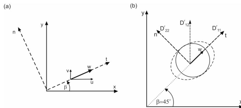
**Figure 3.** (a) Rotation of the  $x$ - $y$  coordinate system by the angle  $\beta$  ( $n$ —perpendicular direction,  $t$ —tangential direction,  $w$ —velocity vector); (b) components of the diffusivity tensor  $D^r$  in the new system  $t$ - $n$  oriented at the angle  $\beta = 45^\circ$ .
