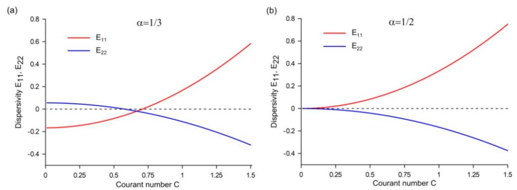
**Figure 4.** The values of the dispersivity tensor components  $E_{11}$  and  $E_{22}$  versus the Courant number  $C$  calculated using the 6N mesh structure for: (a)  $\alpha = 1/3$ ; (b)  $\alpha = 1/2$ .
