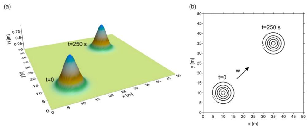
**Figure 7.** Initial condition ( $t = 0$ ) and exact solution ( $t = 250 \text{ s}$ )—the initial wave is only advected along the diagonal with the constant velocity  $w$ : (a) water surface elevation; (b) isolines.
