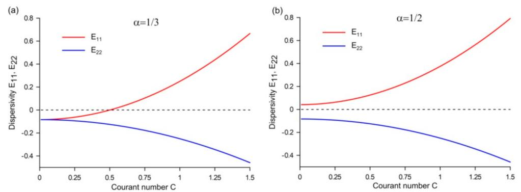
**Figure 6.** The values of the dispersivity tensor components  $E_{11}$  and  $E_{22}$  versus the Courant number  $C$  calculated using the 8N mesh structure for: (a)  $\alpha = 1/3$ ; (b)  $\alpha = 1/2$ .
