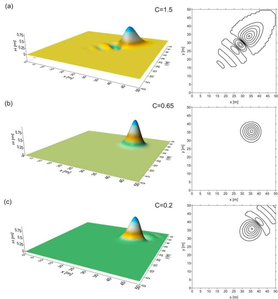
**Figure 9.** Solution obtained using the 6N mesh with  $\theta = 1/2$  and  $\alpha = 1/3$  for various values of the Courant number: (a)  $C = 1.5$ ; (b)  $C = 0.65$ ; (c)  $C = 0.2$ .
