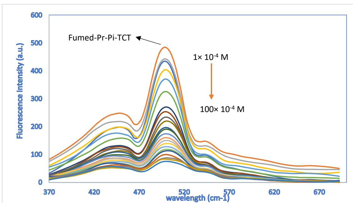
**Figure 6.** Fluorescence response of fumed-Pr-Pi-TCT (3 mL H<sub>2</sub>O suspension, 0.2 g L<sup>-1</sup>) after adding different concentrations of CN<sup>-</sup>.
