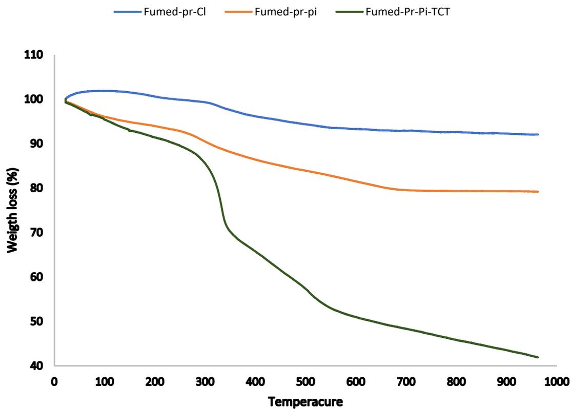
Figure 2. TGA curves of fumed-Pr-Cl, fumed-Pr-Pi, and fumed-Pr-Pi-TCT.
