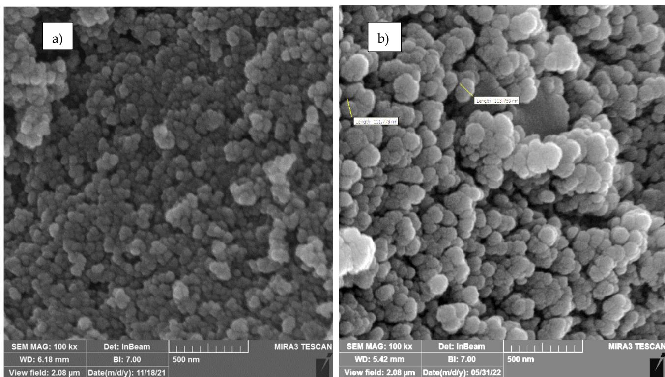
**Figure 3.** SEM images of (a) fumed silica and (b) fumed-Pr-Pi-TCT.
