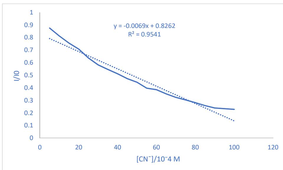
**Figure 7.** Stern–Volmer plot for the titration of fumed-Pr-Pi-TCT with different concentrations of CN<sup>-</sup>.
