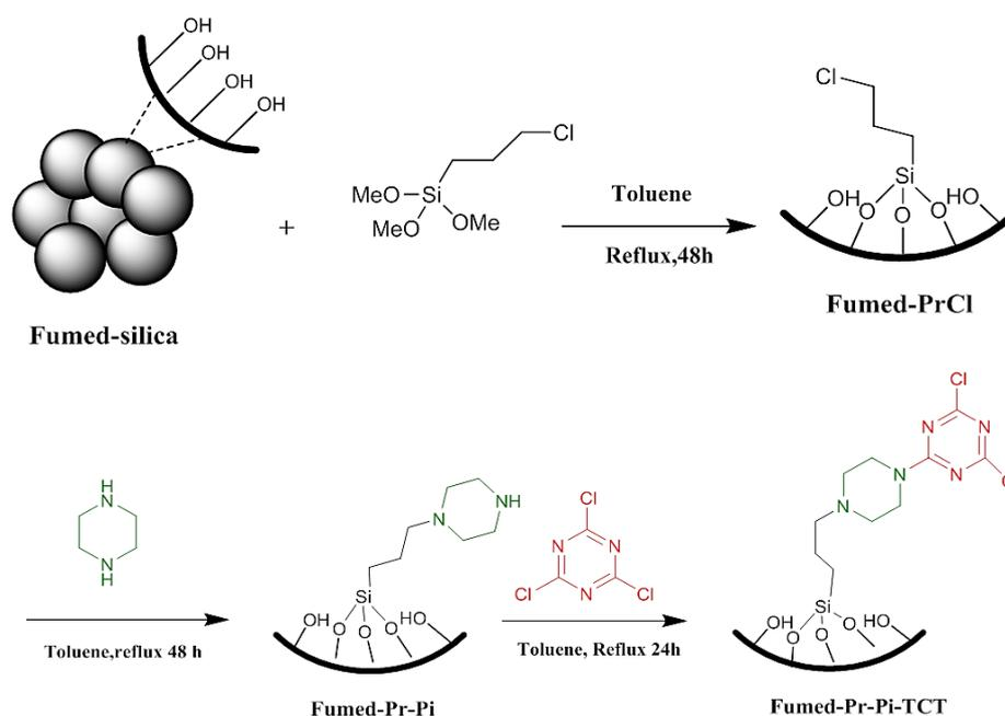
**Scheme 1.** Preparative process for fumed-Pr-Pi-TCT chemosensor.
