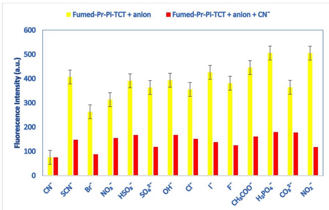
**Figure 5.** Selectivity of fumed-Pr-Pi-TCT (3 mL H<sub>2</sub>O suspension, 0.2 g L<sup>-1</sup>) for CN<sup>-</sup> (100 μL, 1 × 10<sup>-2</sup> M) with equal amounts of interfering anions ( $\lambda_{\text{em}} = 500 \text{ nm}$ ,  $\lambda_{\text{ex}} = 350 \text{ nm}$ ).
