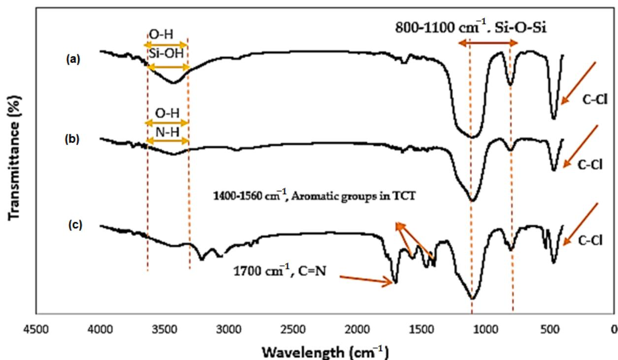
Figure 1. FT-IR analysis of (a) fumed-Pr-Cl, (b) fumed-Pr-Pi, and (c) fumed-Pr-Pi-TCT.
