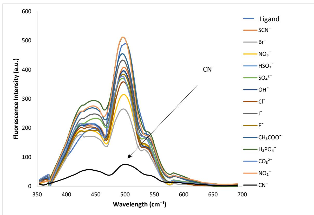
**Figure 4.** Fluorescence spectra of the aqueous suspended fumed-Pr-Pi-TCT (3 mL H<sub>2</sub>O suspension, 0.2 g L<sup>-1</sup>) using different anions.
