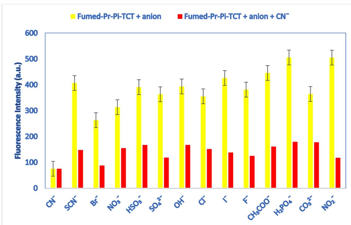
**Figure 5.** Selectivity of fumed-Pr-Pi-TCT (3 mL H<sub>2</sub>O suspension, 0.2 g L<sup>-1</sup>) for CN<sup>-</sup> (100  $\mu$ L,  $1 \times 10^{-2}$  M) with equal amounts of interfering anions ( $\lambda_{em} = 500$  nm,  $\lambda_{ex} = 350$  nm).
