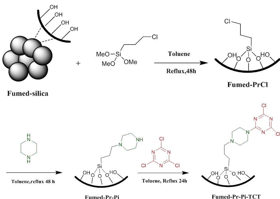
**Scheme 1.** Preparative process for fumed-Pr-Pi-TCT chemosensor.
