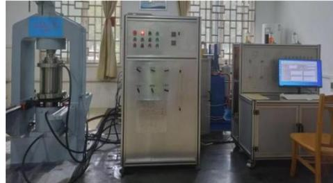
**Figure 3.** The automatic rock triaxial test system.
