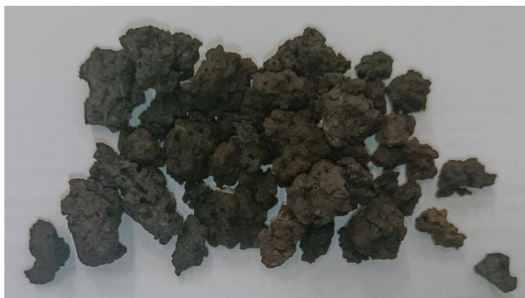
**Figure 1.** Image of biochar obtained by pyrolysis of a sludge–margin mixture at 500 °C.
