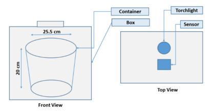
Figure 4. The experimental design to set up the shrimp counting system.
