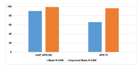
**Figure 12.** Results of mAP when AP = 0.50 and AP 0.75 for the training dataset for default and improved Mask R-CNN.
