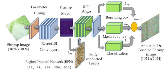
Figure 3. Algorithm for improved Mask R-CNN with parameters calibration step.
