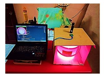
Figure 5. The real view of the experimental setup for the shrimp counting system.
