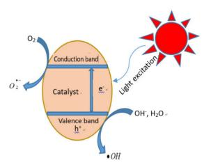
**Figure 4.** Generation of free radicals during photocatalytic reactions.
