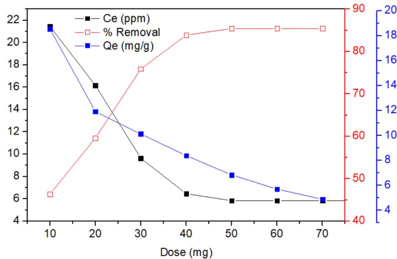
**Figure 7.** Effect of adsorbent dose on the adsorption of RhB.
