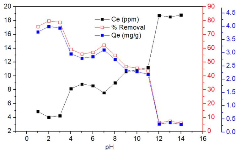
**Figure 3.** Effect of pH on adsorption of RhB dye under experimental conditions, i.e., 10 mL of aqueous solution of RhB (20 ppm), 40 mg of adsorbent, and a contact time of 70 min.
