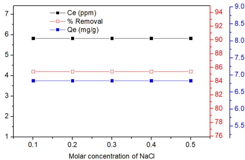
**Figure 4.** Effect of ionic strength on the adsorption of RhB by *C. lawsoniana* at pH 2, 40 ppm RhB, 50 mg of adsorbent, and a contact time of 105 min.
