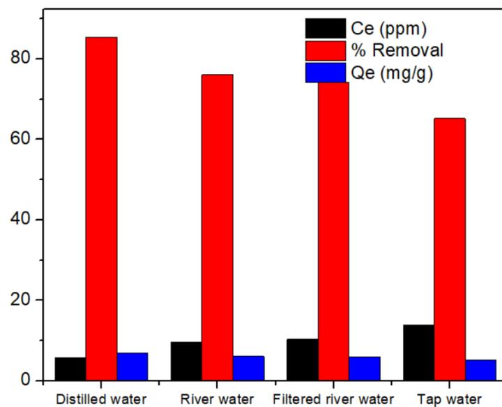
**Figure 8.** Comparative analysis of the adsorbent's efficiency in real water samples at 10 mL of 40 ppm dye solution, pH 2, a contact time of 105 min, and an adsorbent dose of 50 mg.
