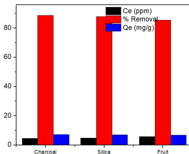
**Figure 9.** Comparative analysis of the adsorption efficiency of dried powdered fruit of *C. lawsoniana*, animal charcoal, and silica gel at 10 mL of 40 ppm dye solution, pH 2, a contact time of 105 min, and an adsorbent dose of 50 mg.
