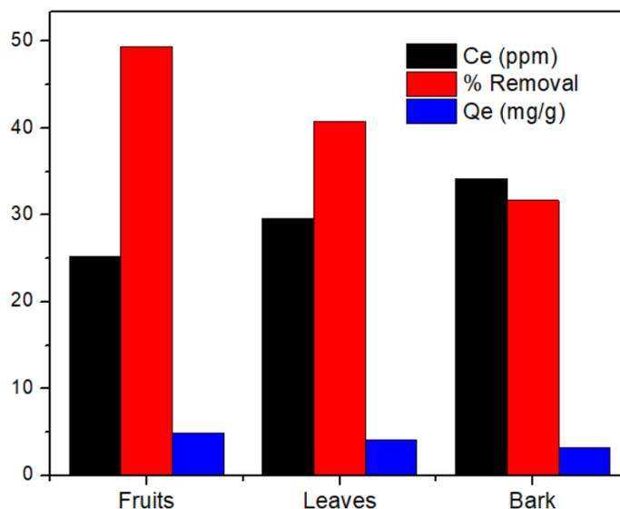
**Figure 2.** Comparison of different parts of *C. lawsoniana* in terms of  $C_e$ ,  $Q_e$ , and % RhB removal at 10 mL of RhB (50 ppm), 50 mg of adsorbent, and a contact time of 70 min.
