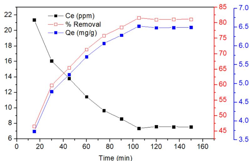
**Figure 6.** Effect of contact time between adsorbent and adsorbate on the adsorption of RhB at experimental conditions such as 10 mL of 40 ppm solution of RhB and 50 mg of adsorbent at pH 2.
