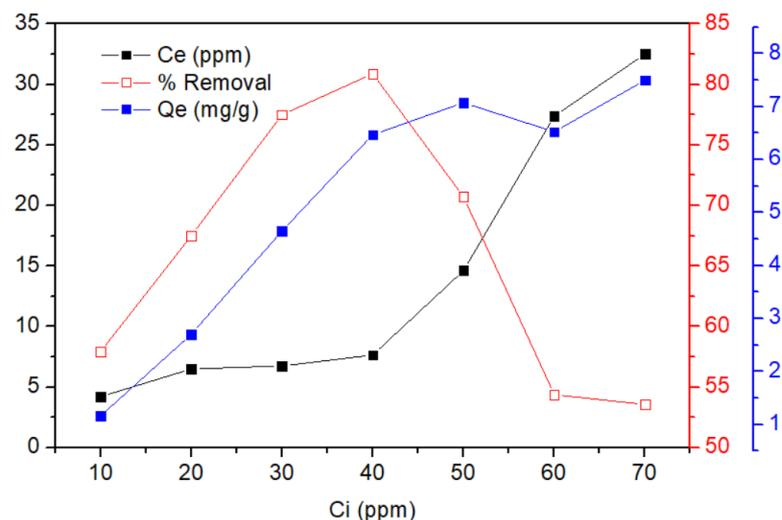
**Figure 5.** Effect of initial concentration of dye on the adsorption parameters at 10 mL solution of RhB (10–70 ppm), 50 mg of adsorbent, a contact time of 70 min, and a pH of 2.
