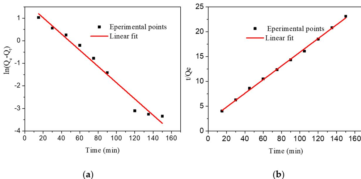
**Figure 10.** Plots of the (a) pseudo-1st-order, and (b) pseudo-2nd-order kinetics models for RhB dye adsorption onto *C. lawsoniana* fruit under experimental conditions such as 10 mL of 40 ppm solution of RhB, 50 mg adsorbent at pH 2.
