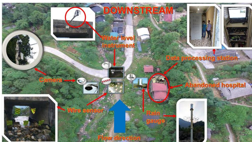
Figure 12. Downstream of the real-time landslide monitoring station.
