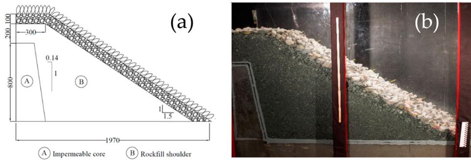
**Figure 6.** (a) Depiction of experimental setup of half dam model with core and (b) image of dumped riprap model with such setup from [26].
