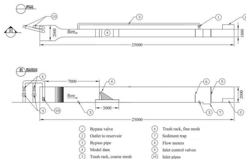
**Figure 3.** Representation of the flume present at the hydraulic laboratory of NTNU (Trondheim) used for the 9 setups introduced in this work. Modified from Kiplesund et al. [22].
