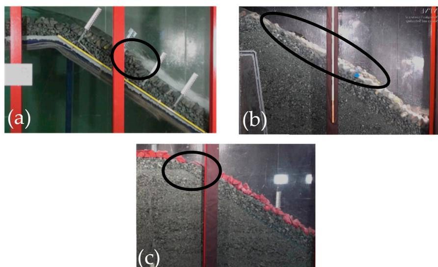
**Figure 9.** Image of the possible failure mechanisms from all tests with (a) buckling (b) sliding and (c) surface erosion mechanisms.
