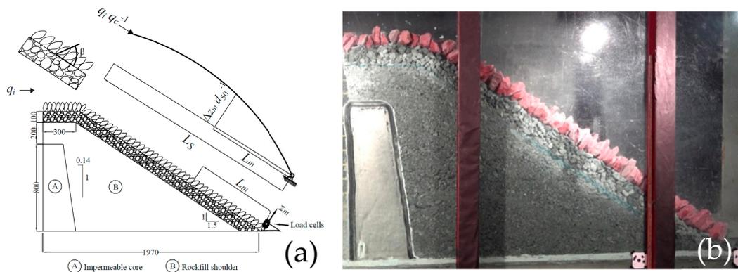
**Figure 7.** (a) Depiction of experimental setup of half dam model with core and placed riprap supported at the toe and (b) image of the model built in the flume.
