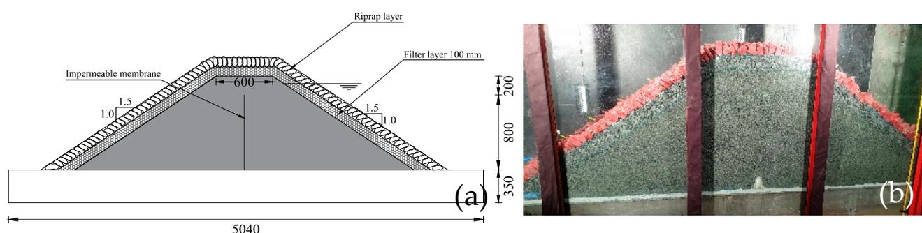
**Figure 8.** (a) Depiction of experimental setup of full dam model with flexible core, and (b) image of placed riprap model with such a setup.
