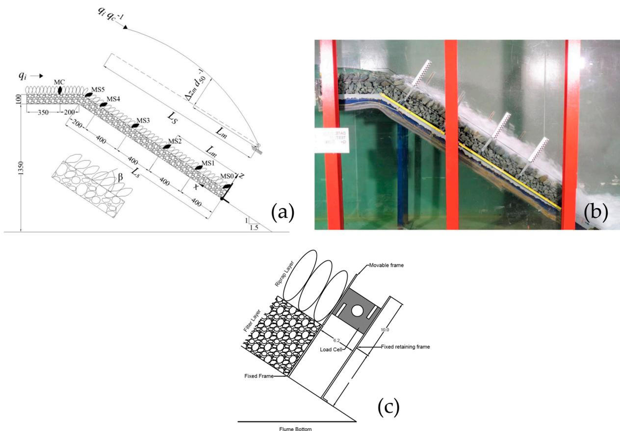
**Figure 4.** From Ravindra et al. [24], (a) depiction of experimental set-up of riprap model supported at the toe, (b) image of placed riprap model with such setup and (c) toe support positioning, from [25].
