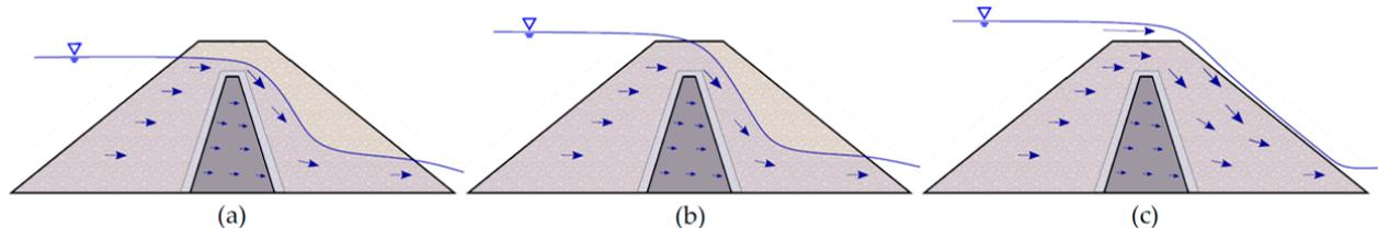
**Figure 2.** (a) Overtopping of the core with throughflow. (b) Partial overtopping of the crest with throughflow. (c) Complete overtopping of the crest with throughflow and overflow of rockfill dams. Modified from [10].
