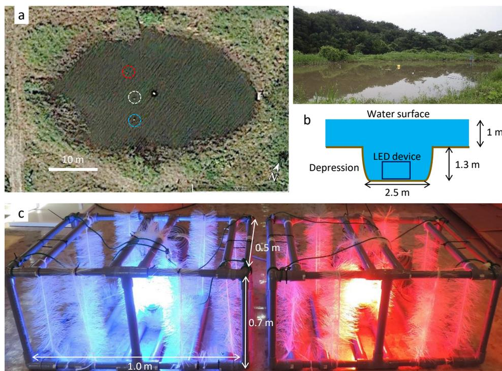
**Figure 1.** Overview of the experimental pond and the location of three depressions (a), vertical view of the depressions (b), and LED devices (blue and red) (c).
