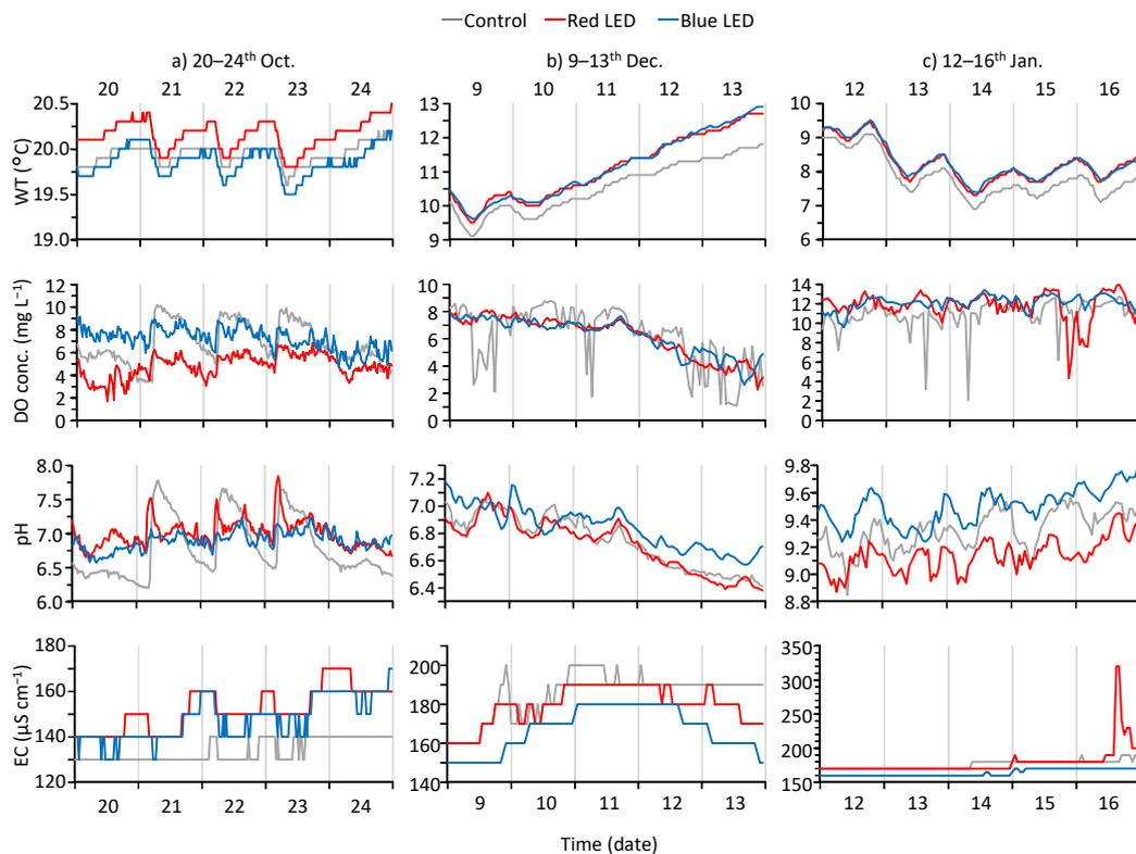
**Figure 4.** Hourly changes in water quality (water temperature, DO, pH, and EC) of the 3 depressions for 5 days ((a): 20–24 October, (b): 9–13 December, (c): 12–16 January).
