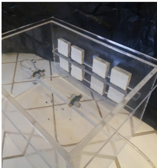
**Figure 1.** Custom-made acid spraying chamber equipped with nebulizers, spraying the surface of coated concrete specimens with the sulfuric acid solution (0.2 M).
