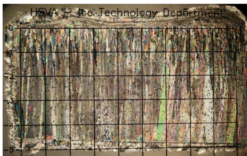
Figure 2. Thin section of model ice.
