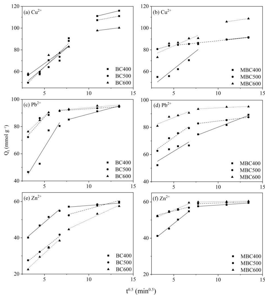
**Figure S3.** Intraparticle diffusion plots of adsorption for  $\text{Cu}^{2+}$  (a,b),  $\text{Pb}^{2+}$  (c,d) and  $\text{Zn}^{2+}$  (e,f) on BCs and MBCs.
