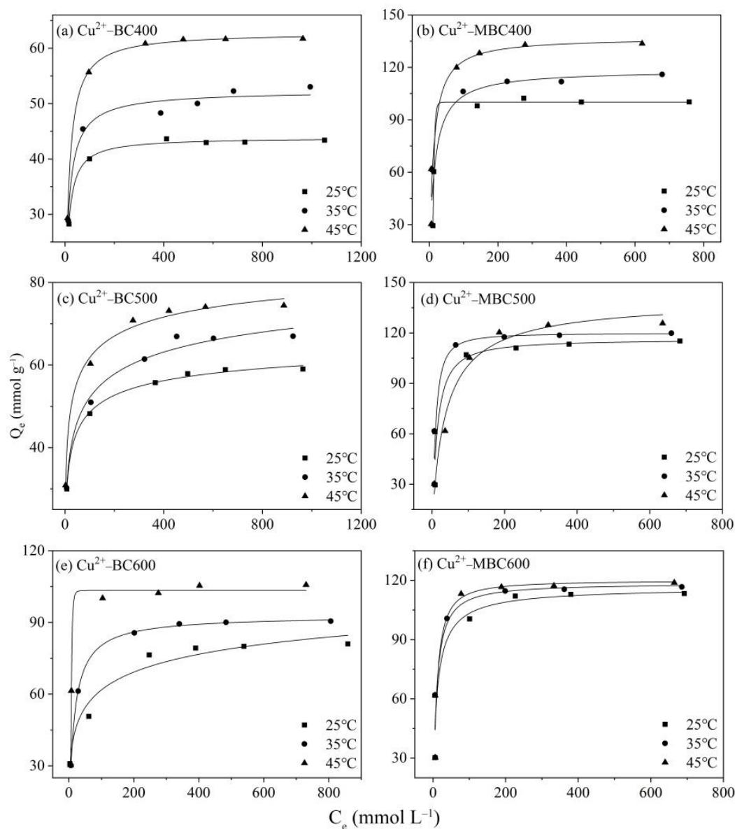
**Figure S4.** Adsorption thermodynamics of  $\text{Cu}^{2+}$  on BCs (a,c,e) and MBCs (b,d,f).
