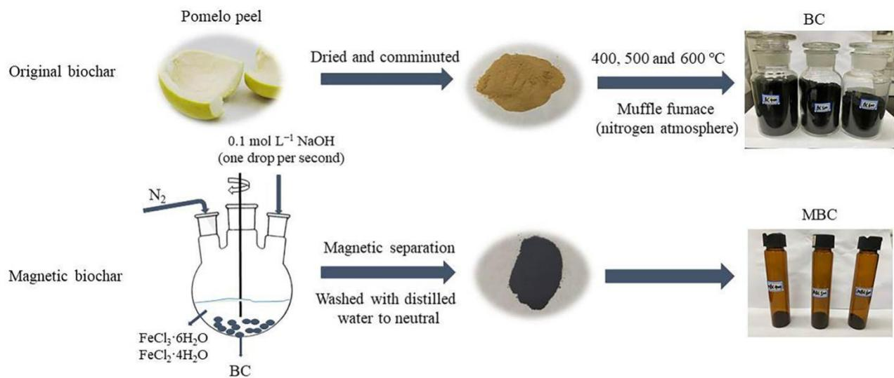
**Figure S1.** Preparation of biochars (BC: biochar, MBC: magnetic biochar).
