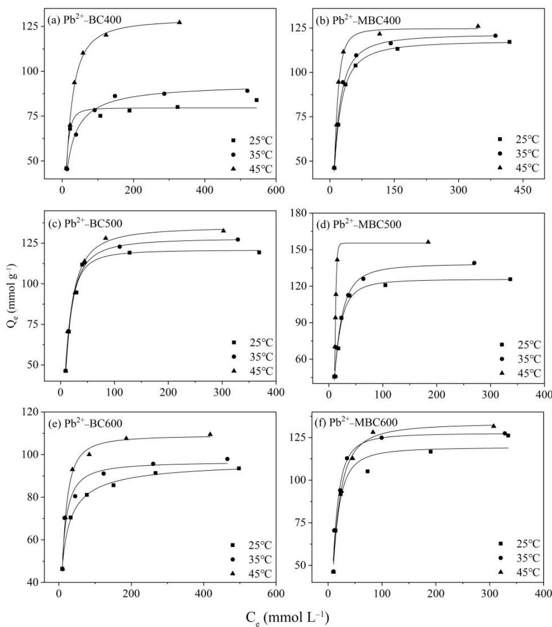
**Figure S5.** Adsorption thermodynamics of  $\text{Pb}^{2+}$  on BCs (a,c,e) and MBCs (b,d,f).
