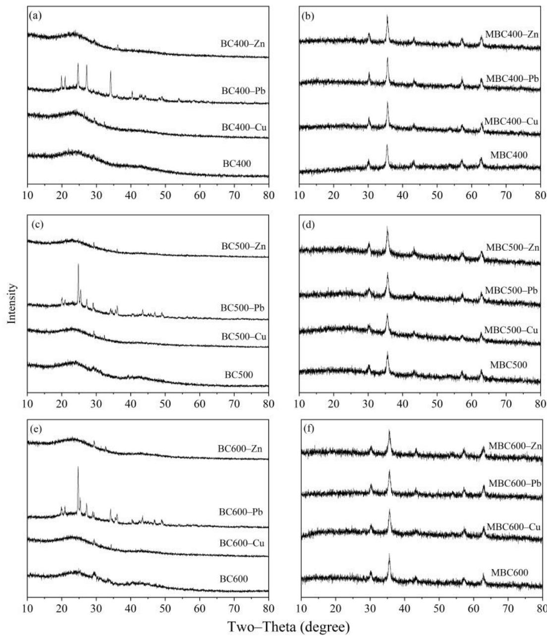
**Figure S8.** XRD patterns of BCs (a,c,e) and MBCs (b,d,f) before and after adsorption of  $\text{Cu}^{2+}$ ,  $\text{Pb}^{2+}$  and  $\text{Zn}^{2+}$ .
