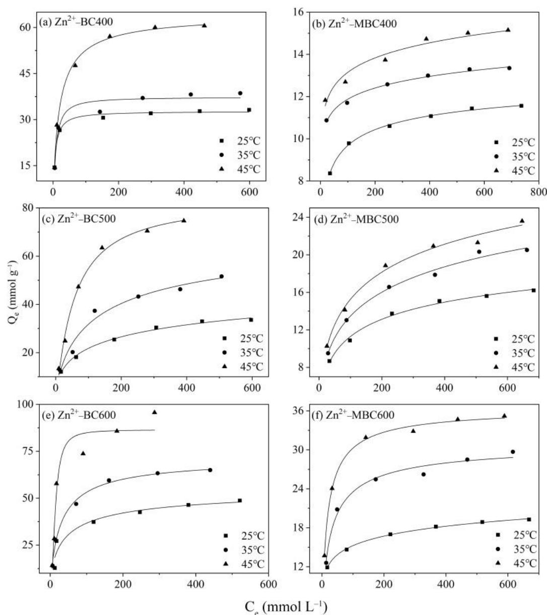
**Figure S6.** Adsorption thermodynamics of  $\text{Zn}^{2+}$  on BCs (a,c,e) and MBCs (b,d,f).
