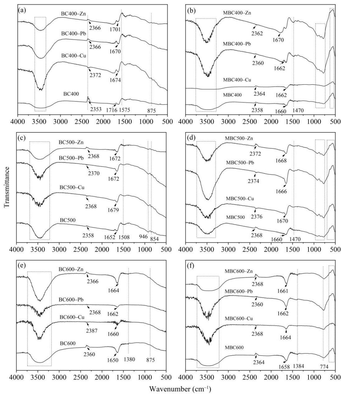
**Figure S7.** FTIR spectra of BCs (a,c,e) and MBCs (b,d,f) before and after adsorption of  $\text{Cu}^{2+}$ ,  $\text{Pb}^{2+}$  and  $\text{Zn}^{2+}$ .
