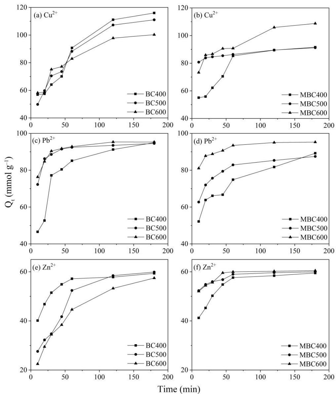
**Figure S2.** Adsorption kinetics of  $\text{Cu}^{2+}$  (a,b),  $\text{Pb}^{2+}$  (c,d) and  $\text{Zn}^{2+}$  (e,f) on BCs and MBCs.
