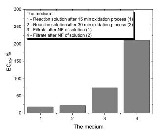
**Figure 9.** Toxicity tests of solution tetracycline hydrochloride (TRC) and its oxidation products (Ops) during oxidation by  $UV/H_2O_2$  exposition time 48 h.
