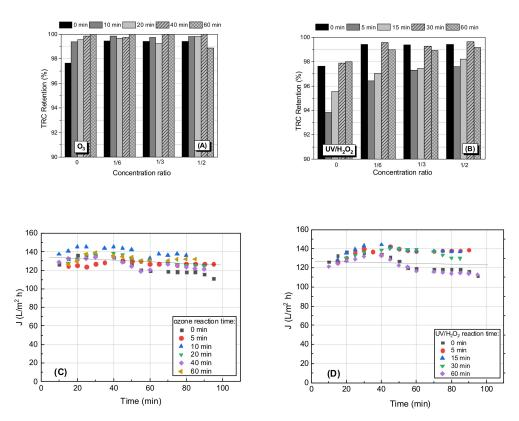
**Figure 4.** (**A**) TRC retention for different reaction time of ozonation; (**B**) TRC retention for different reaction time of  $UV/H_2O_2$ ; (**C**) filtrate flux (J) for nanofiltration of ozonated TRC solution; (**D**) filtrate flux for nanofiltration of  $UV/H_2O_2$ —oxidized TRC solution; membrane HL; pressure 1.0 MPa; temp. 30 °C.
