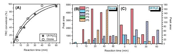
**Figure 2.** (**A**) Dependence of TRC conversion on oxidation time (for ozone and  $UV/H_2O_2$ ); (**B**) Peak area of the identified products during ozonation; (**C**) Peak area of the identified products during  $UV/H_2O_2$  treatment.
