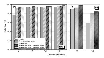
**Figure 10.** (**A**) The filtrate flux for a different water matrix with dissolved TRC; (**B**) TRC retention for different water matrix; (**C**) P6 retention for different water matrix.
