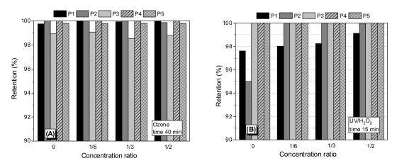
Figure 6. Ops retention (A) for 40 min of ozonation; (B) for 15 min of UV/H<sub>2</sub>O<sub>2</sub> oxidation; membrane HL.
