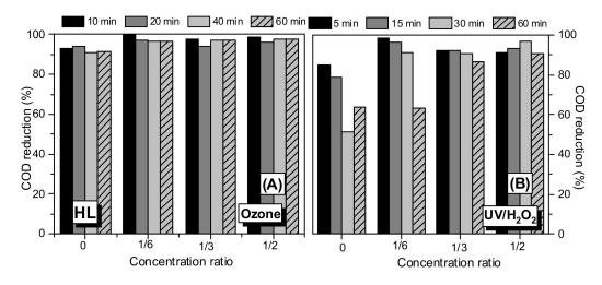
Figure 7. Chemical oxygen demand COD reduction during NF of oxidized TRC solution: (A) after ozonation; (B) after UV/H<sub>2</sub>O<sub>2</sub>.
