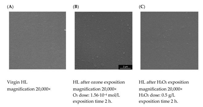
Figure 5. SEM pictures of the HL membrane: (A) virgin HL; (B) HL after ozone exposure; (C) HL after  $H_2O_2$  exposure.
