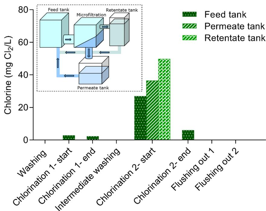
**Figure 6.** Concentration of free chlorine in samples acquired from the cleaning process in the food industry. Insert (stipple box): Schematic of a membrane system and flow during recycling of water in the cleaning process.
