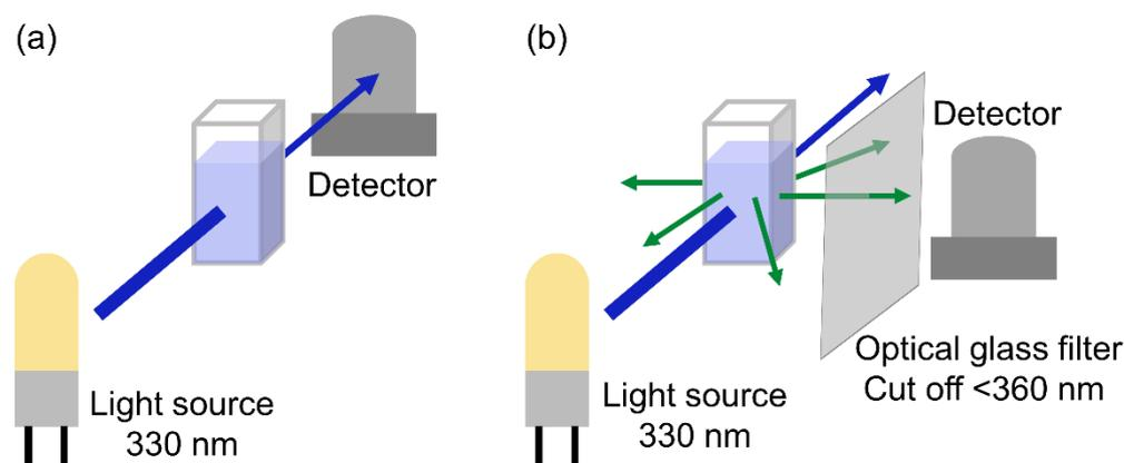
**Figure 7.** Conceptual drawing of the construction of meter for absorbance measurement (a) and fluorescence measurement (b).
