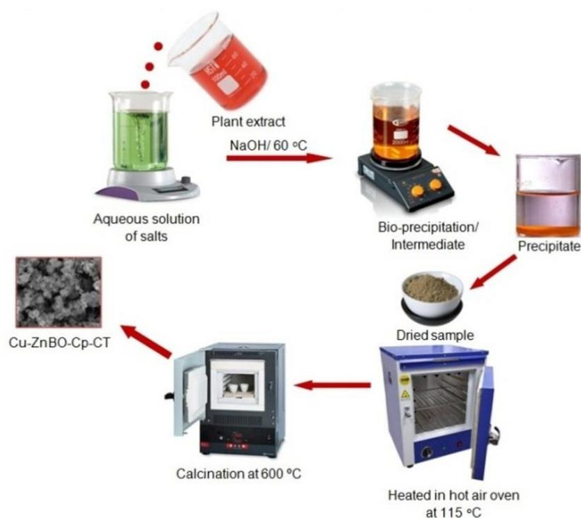
Figure A1. Schematic diagram of preparation of Cu-ZnBO-Cp-CT.
