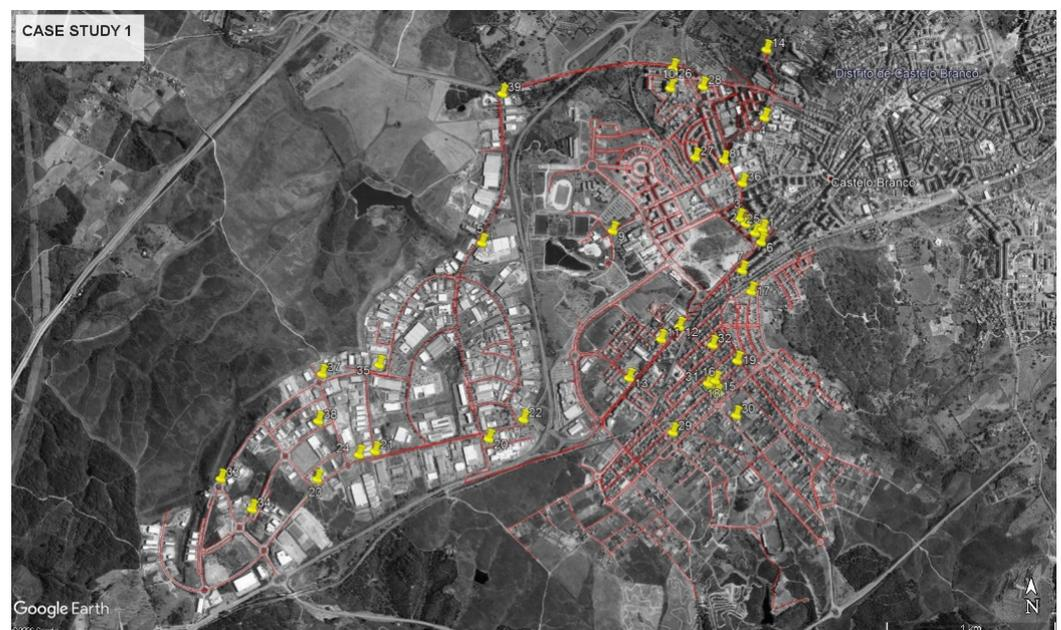
**Figure 3.** Case Study 1 water distribution system and water quality sampling locations.
