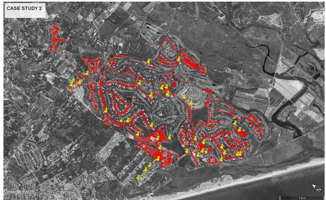
**Figure 4.** Case Study 2 water distribution system and water quality sampling locations.
