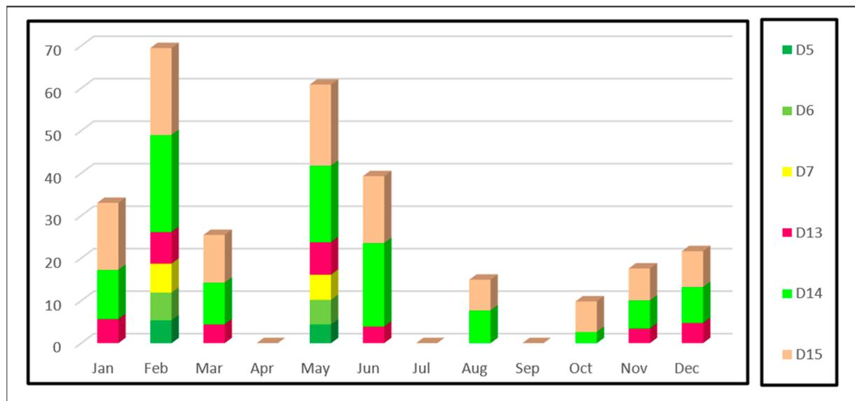
**Figure 14.** Monthly unmet demand (MCM) of lining three sections.
