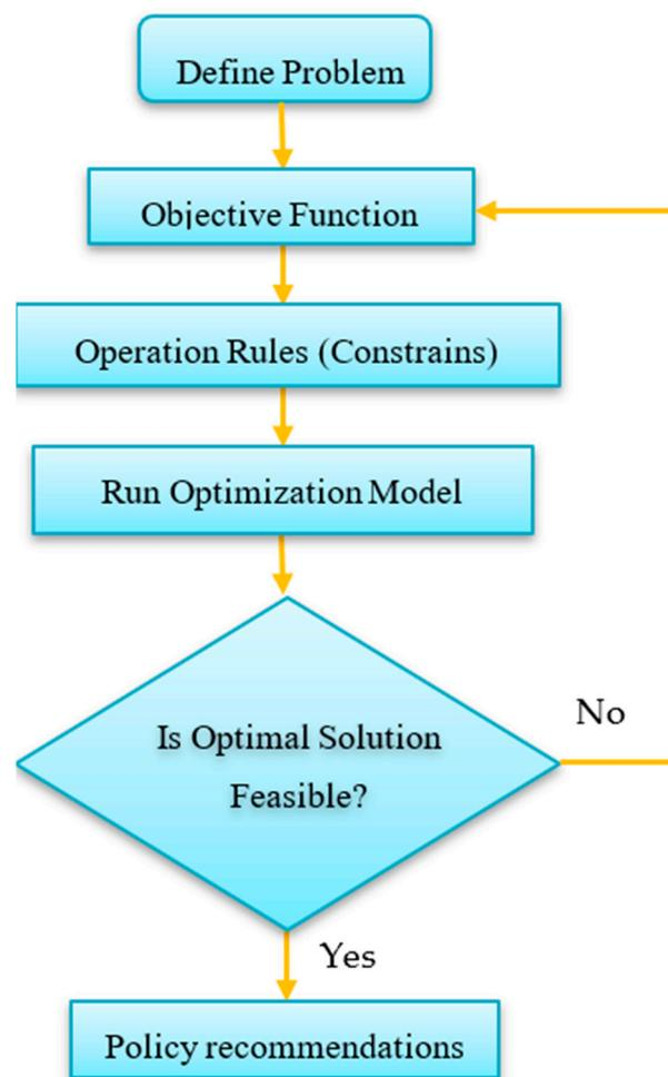
Figure 3. Simplified flowchart for optimization modelling.
