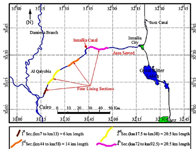
**Figure 13.** Ismailia Canal from its inlet at Cairo until it reaches the Ismailia governorate showing the four lining sections and their length [52].
