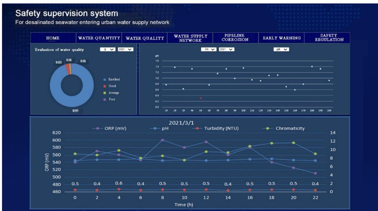
**Figure 4.** On-line monitoring data of ORP, pH, turbidity, and chromaticity.
