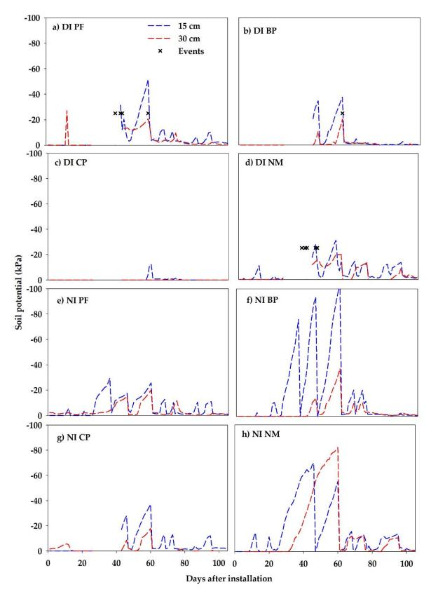
**Figure 3.** Daily average soil matric potential (09:00 am) at 15 and 30 cm deep in tomato plots during 2019 field experiment under drip irrigation (DI) treatment with (**a**) landscape fabric mulch (DI PF), (**b**) black plastic mulch (DI BP), (**c**) clear plastic mulch (DI CP), (**d**) no mulch (DI NM), and no irrigation treatment (NI) with (**e**) landscape fabric mulch (NI PF), (**f**) black plastic mulch (NI BP), (**g**) clear plastic mulch (NI CP), and (**h**) no mulch (NI NM).
