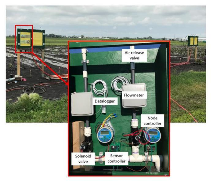
Figure 2. Irrigation controller board with two control units.
