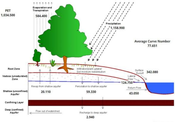
The SWAT Check results from the James River model display the overall hydrologic budget of the watershed for the output period 1988–2018 (Figure A1).
