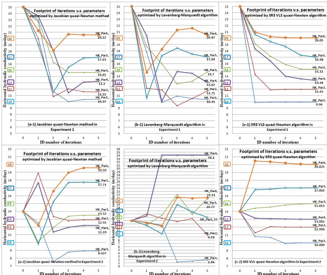
**Figure 2.** Footprint of iterations vs. hydraulic conductivity in Experiment 1 and Experiment 2 optimized by (a) Jacobian quasi-Newton method; (b) LMA; (c) SR3 VLS quasi-Newton algorithm.
