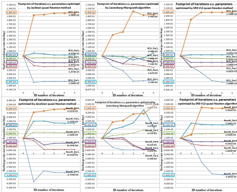
Figure 4. Footprint of iterations vs. surface recharge (-1) and boundary recharge (-2) in Experiment 2 optimized by (a) Jacobian quasi-Newton; (b) L-M algorithm; (c) SR3 VLS quasi-Newton algorithm.
