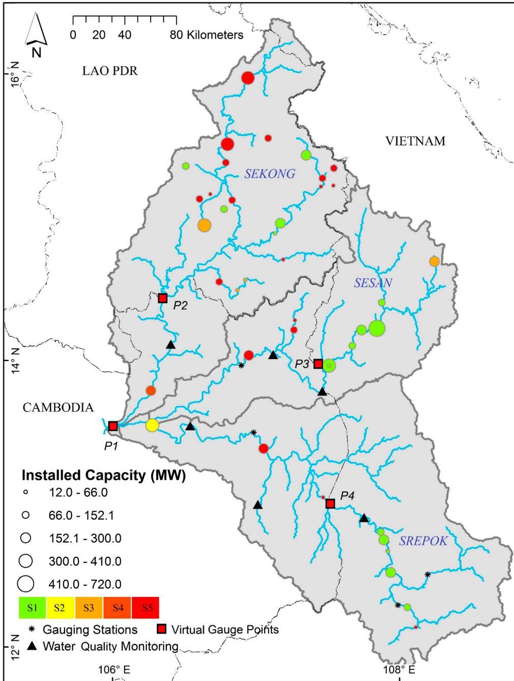
**Figure 1.** The Sesan, Srepok and Sekong basins showing deviation from natural flow assessment locations, flow gauging stations, water quality monitoring stations and the location and capacity of the main dams considered in the five hydropower development scenarios.
