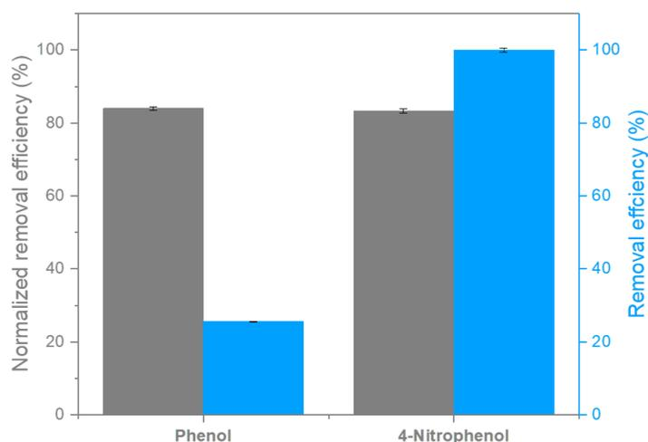
**Figure 1.** Normalized removal efficiency % data to 0–1 range on the maximal value after 4 hours of the uptake process (gray) and removal efficiency % at equilibrium (blue) for an aqueous solution of phenol and 4-nitrophenol.
