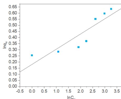
**Figure 2.** Fitting of experimental data with linearized Freundlich isotherm model for phenols in OMW ( $R^2 = 0.8$ ).
