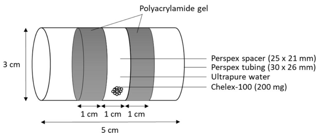
**Figure 2.** The artificial mussel design (Wu et al., 2007).
