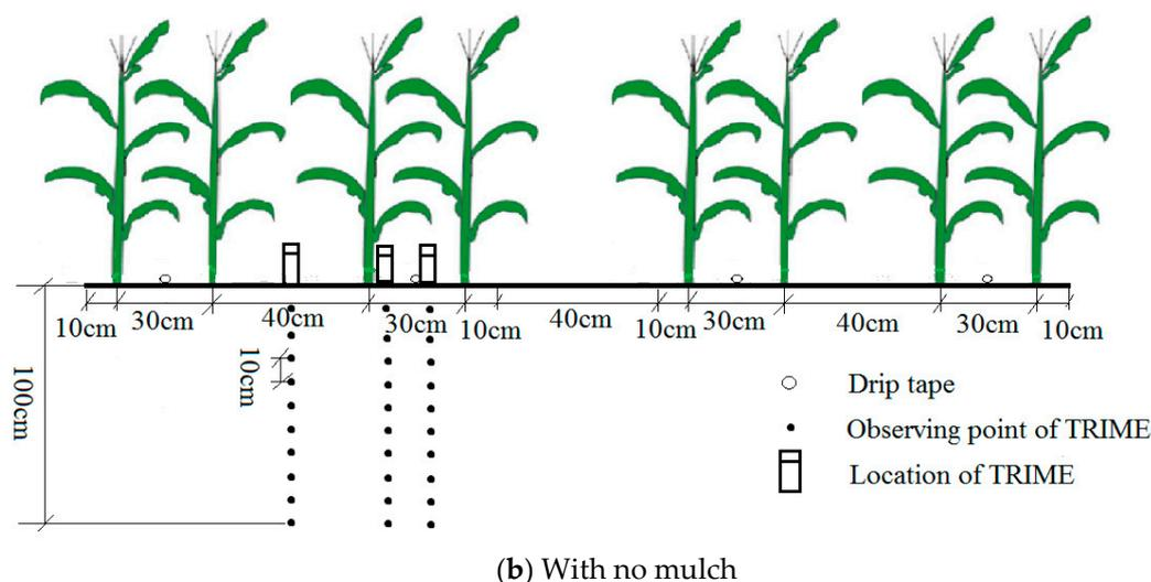
**Figure 1.** Plot design for estimating evapotranspiration of drip-irrigated summer maize in Xinjiang, China. (a) With partial mulch; (b) With no mulch. (TRIME was the TRIME TDR system to determine the soil volumetric water content).
