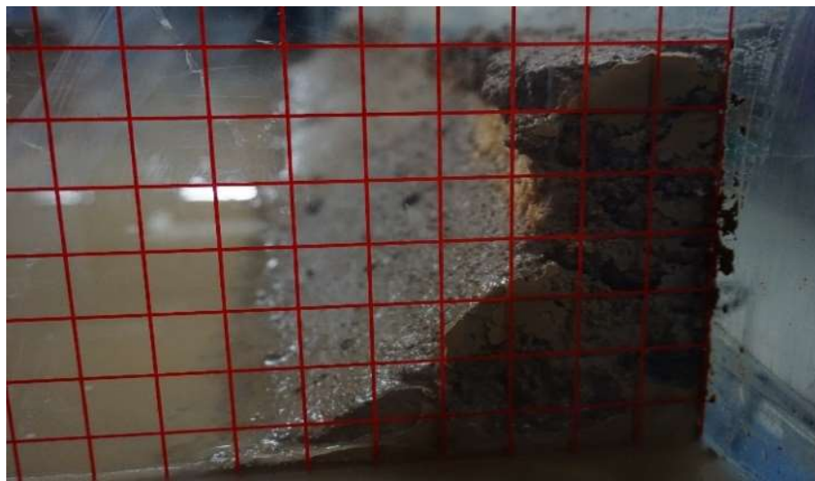
Figure 6. Schematic diagram of a topographical measurement conducted after the collapse section using a system of gridlines.
