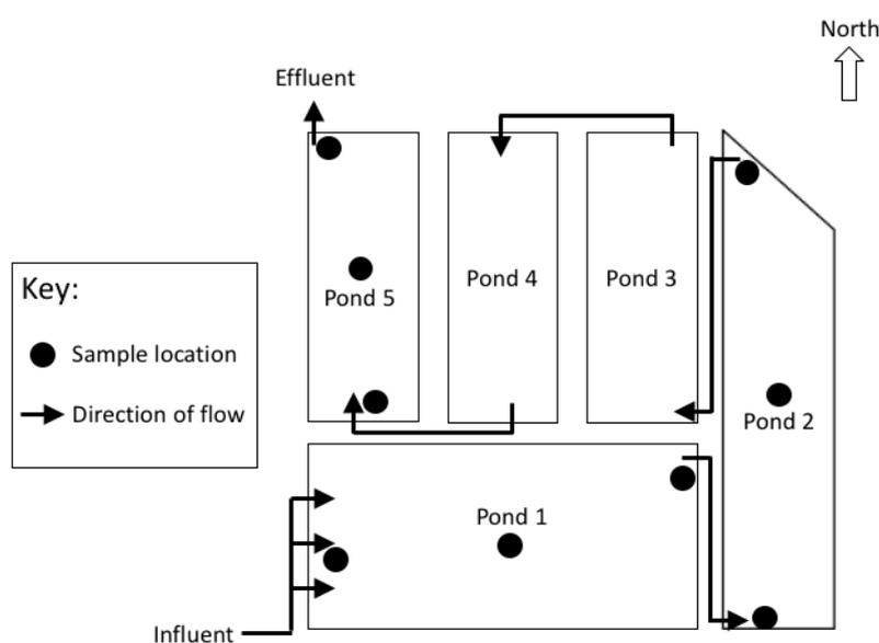
**Figure 1.** Pond schematic showing the sampling locations in facultative (Pond 1), first maturation (Pond 2) and fourth maturation (Pond 5) ponds of the Sanderson waste stabilization ponds (WSP) system. Estimated hydraulic retention times for each pond are: 10 days (Pond 1); 7 days (Pond 2); and 1.5 days (Pond 5).
