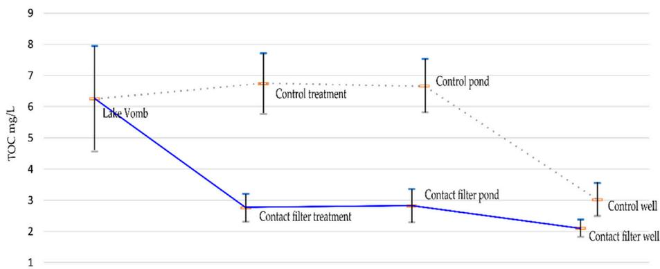
**Figure 4.** Total organic carbon (TOC) measurements at different stages along the two treatment processes (mg/L). The middle bar is the mean value and the top and lower bars show the standard deviation. The dotted line is the contact filter treatment process and the solid line is the control treatment process.
