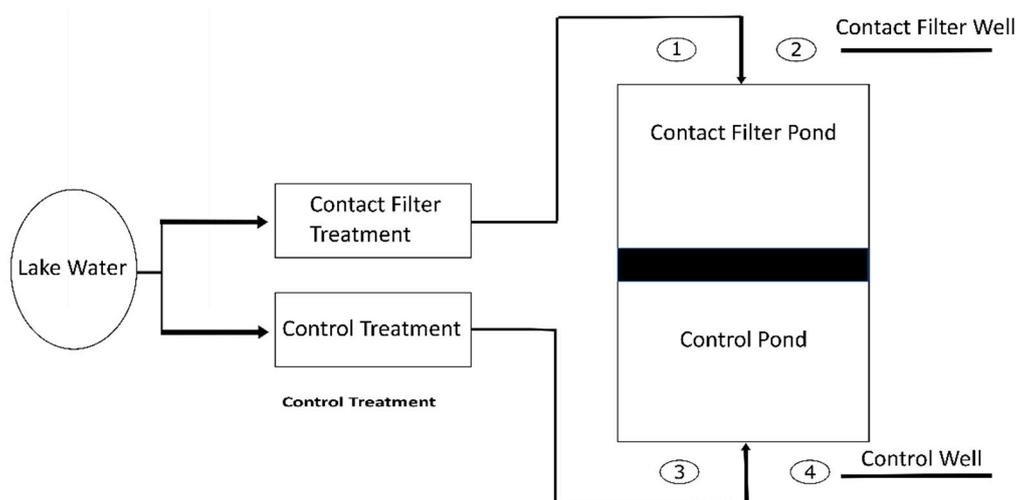
**Figure 1.** Study site overview. The lake is Lake Vomb from which water is led either through contact filter treatment or control treatment to their corresponding pond, i.e., contact filter pond and control pond.
