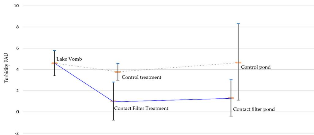
**Figure 2.** Turbidity measurements at different stages along the two treatment processes (FAU). The middle bar is the mean value and the top and lower bars show the standard deviation. The dotted line is the contact filter treatment process and the solid line is the control treatment process.
