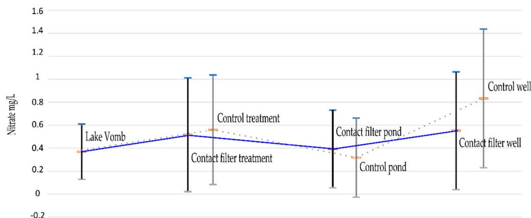
**Figure 6.** Nitrate content at different stages along the two treatment processes (mg/L). The middle bar is the mean value and the top and lower bars show the standard deviation. The dotted line is the contact filter treatment process and the solid line is the control treatment process.
