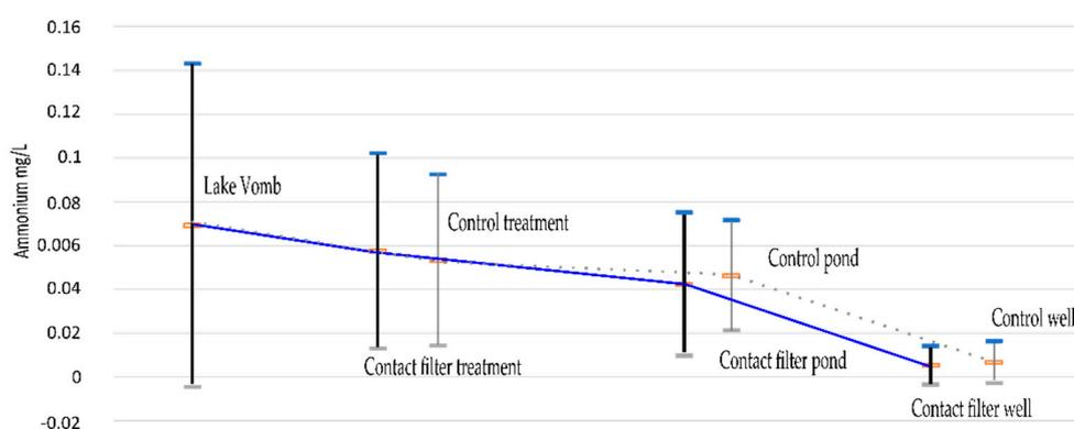
**Figure 7.** Ammonium content at different stages along the two treatment processes (mg/L). The middle bar is the mean value and the top and lower bars show the standard deviation. The dotted line is the contact filter treatment process and the solid line is the control treatment process.
