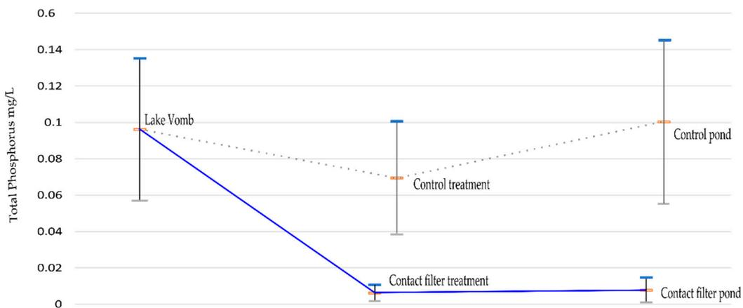
**Figure 5.** Total phosphorus removal at different stages along the two treatment processes. The middle bar is the mean value and the top and lower bars show the standard deviation. The dotted line is the contact filter treatment process and the solid line is the control treatment process.
