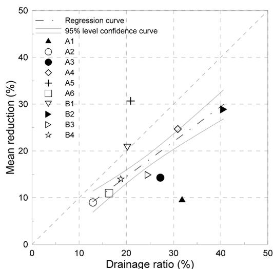
**Figure 7.** Mean runoff reduction by drainage ratio (drainage area of each sub-basin/LID drainage area × 100%) from the short-term simulation.
