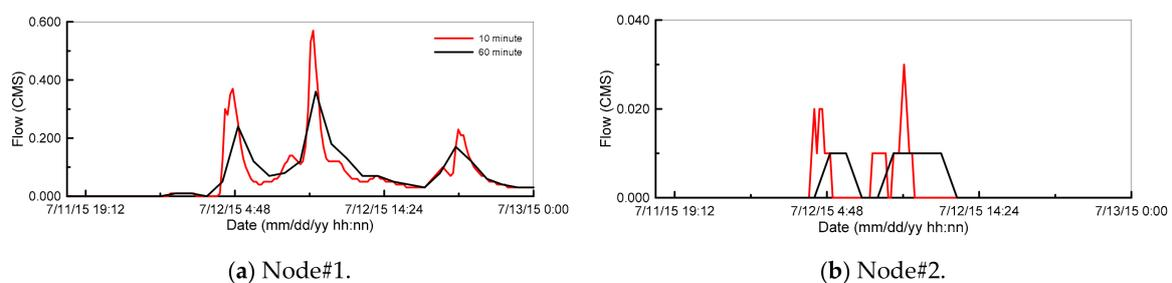
**Figure 4.** Comparisons of runoff simulated from precipitation data for 60-min periods directly recorded (black) and 60-min periods estimated from 10-min data: In this figure, Node# 1 and #2 indicate two of nodes (or junctions) in the SWMM-LID model for the application area. The unit, cms, means a cubic meter per second.
