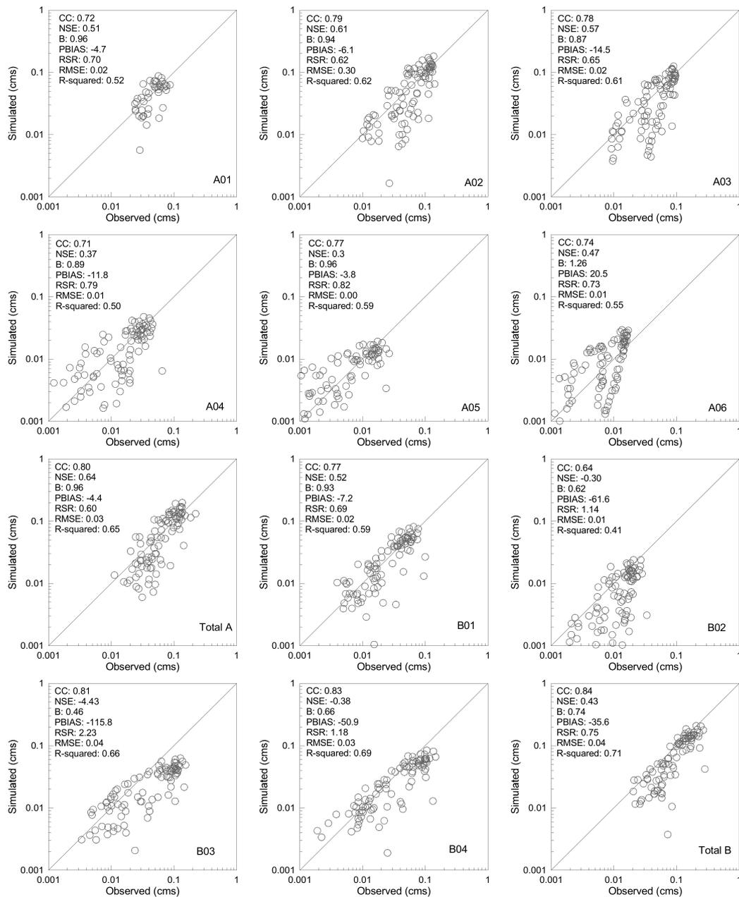
**Figure 5.** Calibration results for each sub-basin of the study area using observed and simulated runoff flows for the E1 and E2 storm events. In this figure, correlation coefficient (CC), Nash-Sutcliffe efficiency coefficient (NSE), Bias (B), percent bias (PBIAS), RMSE-observations standard deviation ratio (RSR), root-mean-square error (RMSE), and R-squared are used as error indices to verify the calibration results.
