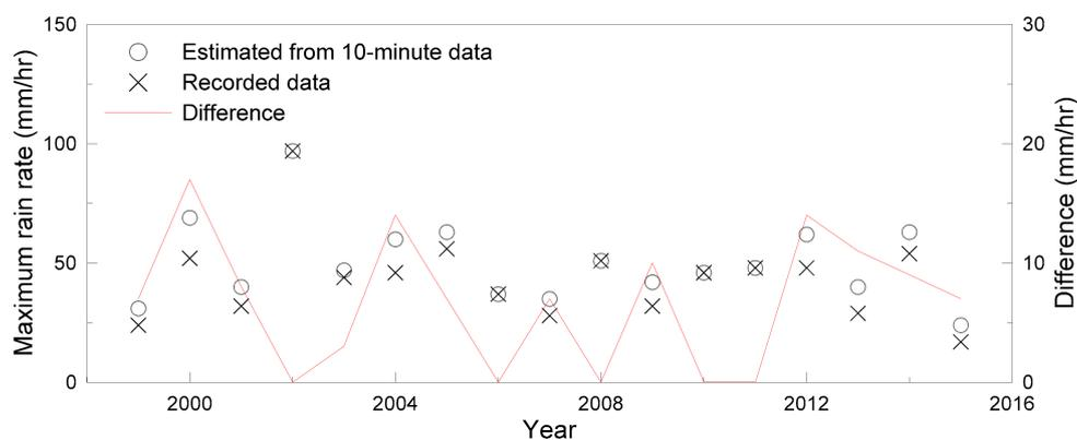
**Figure 3.** The difference (red line) between annual maximum 60-min precipitation as directly recorded (Xs) and that estimated from 10-min precipitation data (Os).
