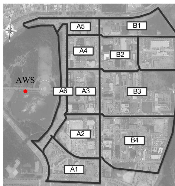
**Figure 1.** Total drainage area of the study site at the Ochang Science Industrial Complex, Cheongju, South Korea, showing the 10 sub-basins considered in this study. In the figure, the red point indicates the nearest automatic weather station (AWS) around the drainage area.
