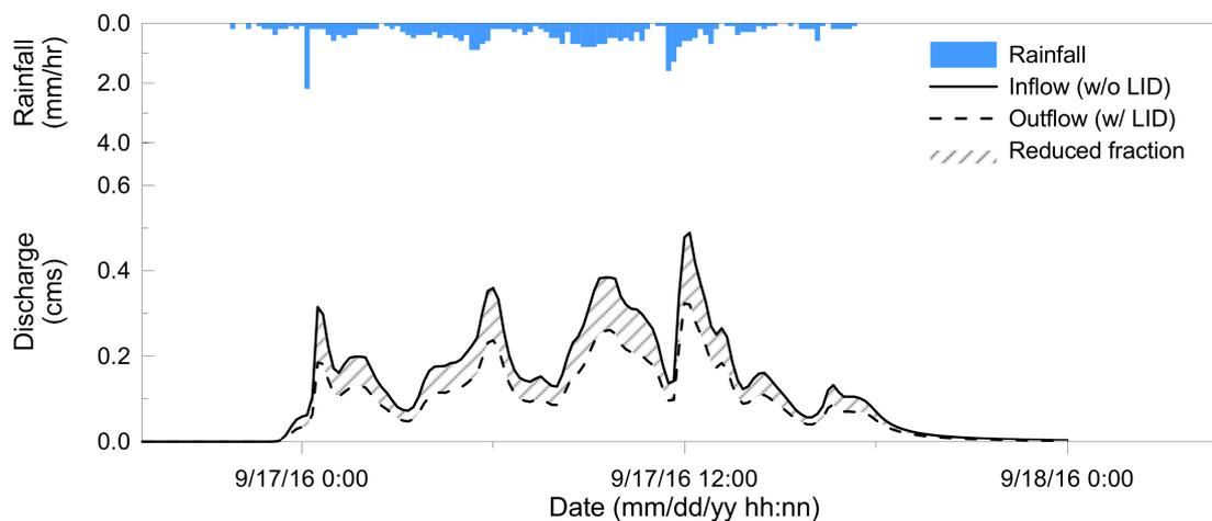
**Figure 6.** Hydrograph results of the total drainage area: In this figure, the hydrograph consists of inflow, outflow, and reduced fraction. The inflow indicates a case without LID facilities and the outflow is the other case with LID facilities. The reduced fraction means a portion of reduced runoff by LID facilities.
