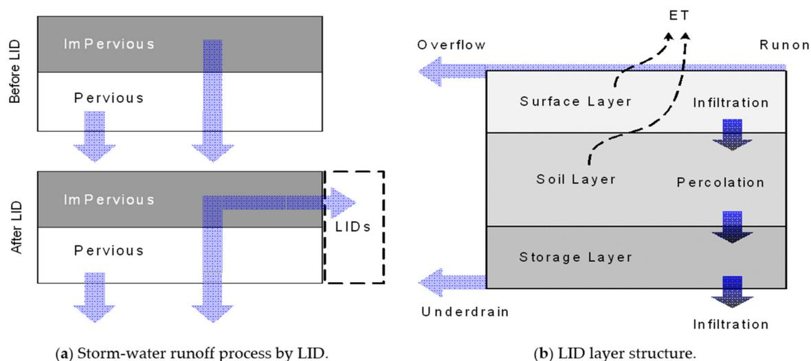
**Figure 2.** Conceptual diagram of the storm-water runoff process by LID facility and LID layer structure in SWMM-LID model [7].
