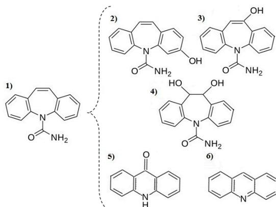
**Figure 4.** Identified 1 carbamazepine by-products, where 2 is 3-hydroxycarbamazepine, 3 is 10,11-dihydro-10-hydroxycarbamazepine, 4 is dihydrocarbamazepine-10,11-trans-diol, 5 is 9-acridone, and 6 is acridine.
