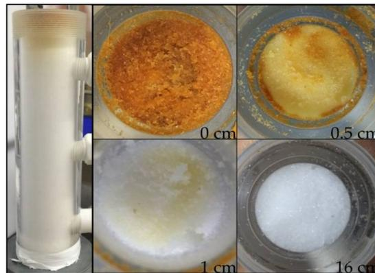
**Figure 9.** Porous matrix iron oxide particles interception for different sections.
