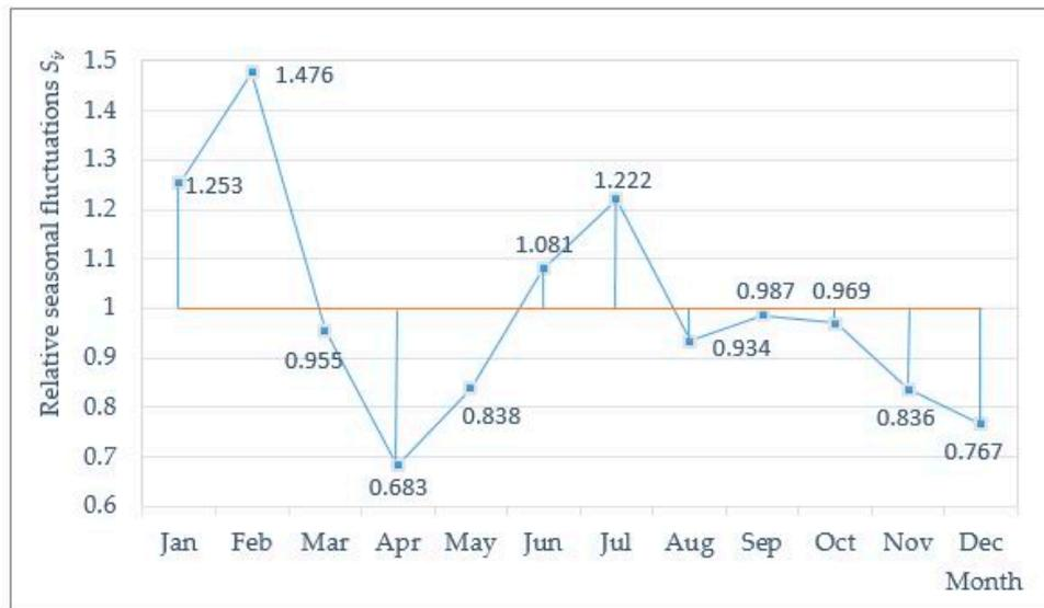
**Figure 7.** Relative seasonal fluctuations of failure rates in WDN.
