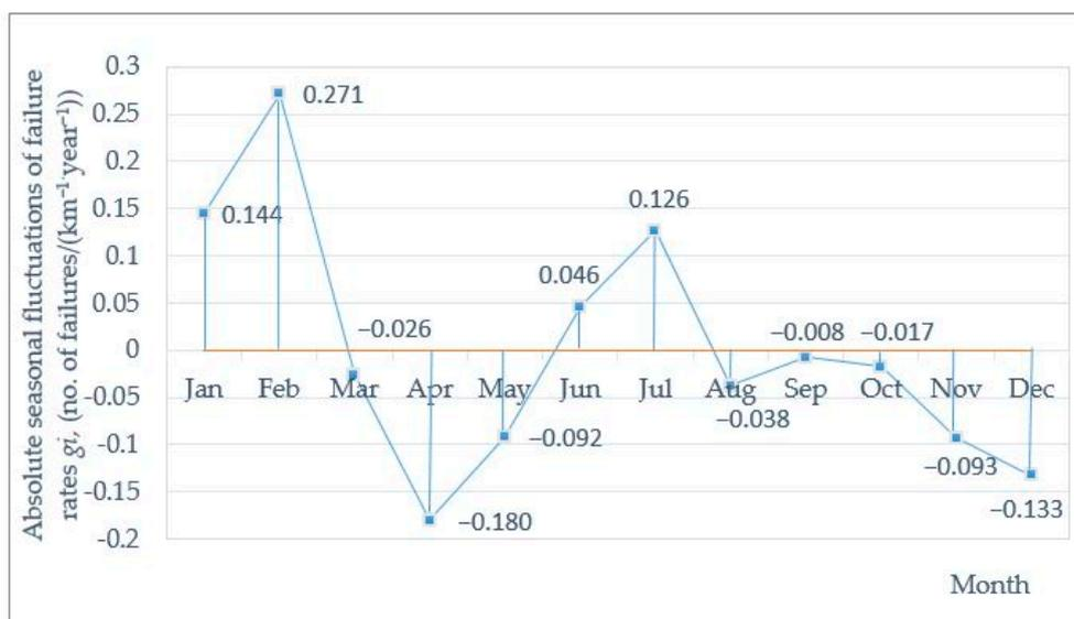
Figure 8. Absolute seasonal fluctuations of failure rates in WDN, in (no. of failures/(km<sup>-1</sup>.year<sup>-1</sup>)).
