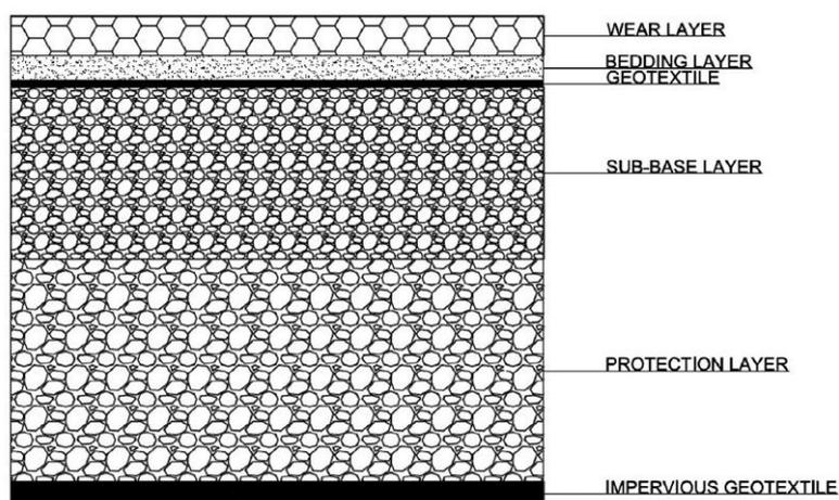
**Figure 5.** Structure of the permeable pavement used in the study. **Source:** Maiolo et al. [9].
