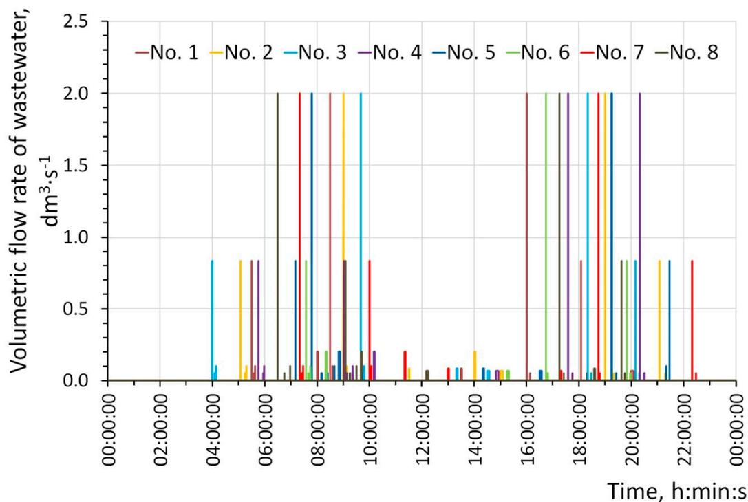
**Figure 9.** Patterns of raw wastewater inflow to ST during 24 h based on data in Table 2.
