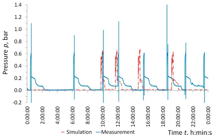
**Figure 14.** Pressures of wastewater in the force main just downstream of PS\_2 measured on 20 October 2016 and simulated for day 3 using the SWMM 5.1.
