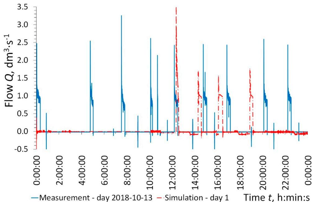
**Figure 11.** Flows in force main measured on 13 October 2016 and simulated for day 1 using the SWMM 5.1 program.
