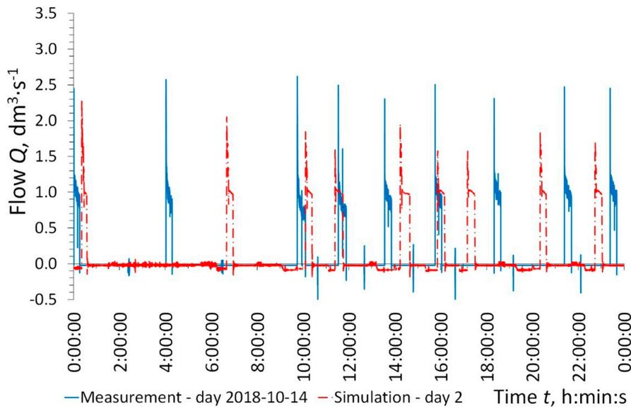
**Figure 12.** Flows in force main measured on 14 October 2016 and simulated for day 2 using the SWMM 5.1 program.
