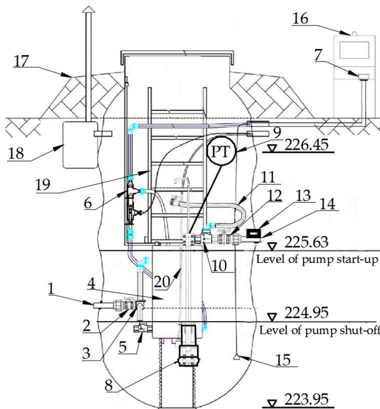
**Figure 4.** Wastewater pumping station PS\_1 according to the design project. Legend: 1—Inlet PE 63 mm; 2—Valve; 3—Check valve; 4—Vacuum tank; 5—Check valve; 6—Float switch for vacuum pump; 7—Vacuum pump; 8—Submersible pump; 9—Pressure transducer; 10—Check valve; 11—Emitter with almost closed valve; 12—Valve; 13—Ultrasonic flowmeter; 14—Outlet; 15—Measuring bell; 16—Control cabinet; 17—Bank; 18—Biofilter; 19—Ladder; 20—Electric cable.
