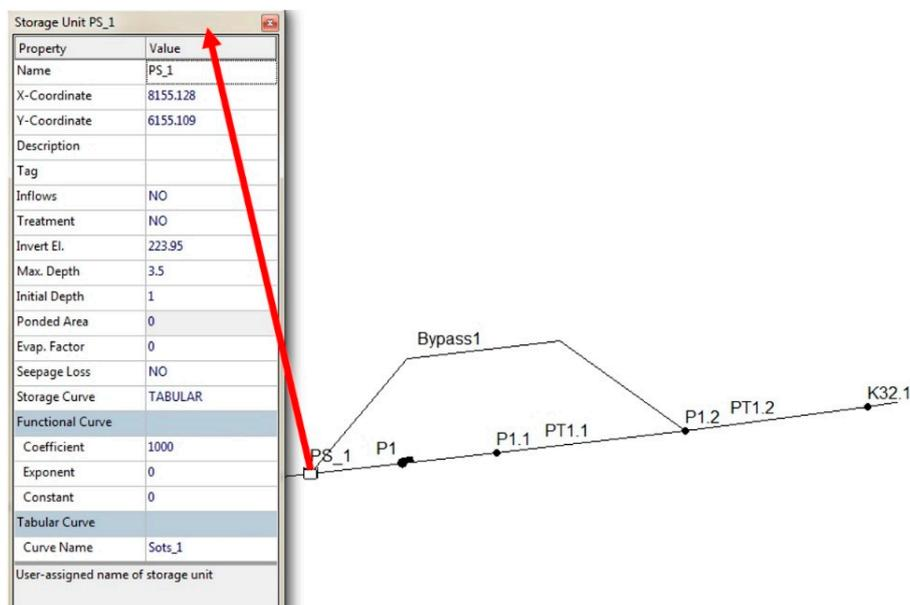
**Figure 8.** View of the storage unit properties editor acting as the pumping station PS\_1.
