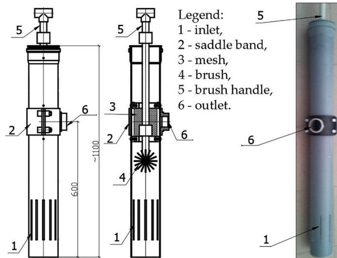
Figure 5. Effluent filter—vertical section and side views.
