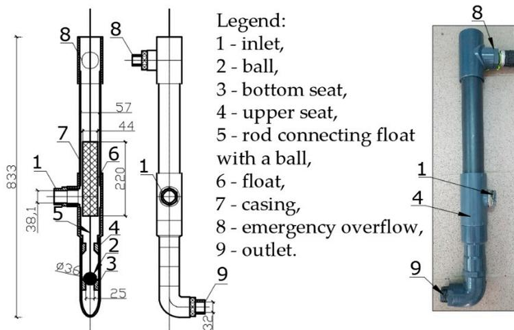
Figure 6. Vertical section and side view of the check valve at the ST outlet.
