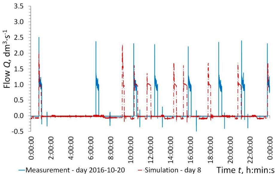
**Figure 13.** Flows in force main measured on 20 October 2016 and simulated for day 8 using the SWMM 5.1 program.
