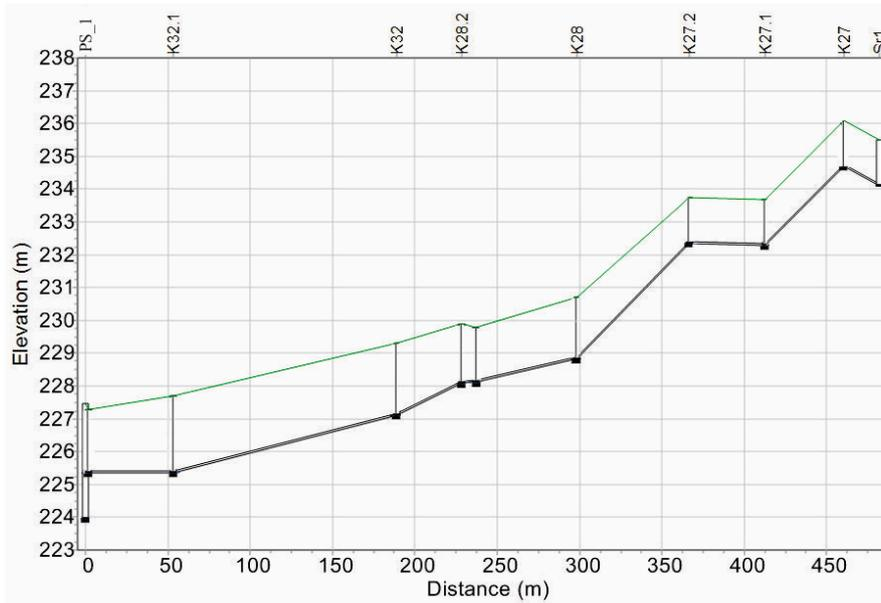
Figure 2. Profile of small diameter gravity sewerage system between pumping stations PS\_2 and PS\_1.
