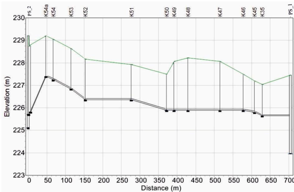
Figure 3. Profile of small diameter gravity sewerage system between pumping station PS\_1 and manhole Sr1.
