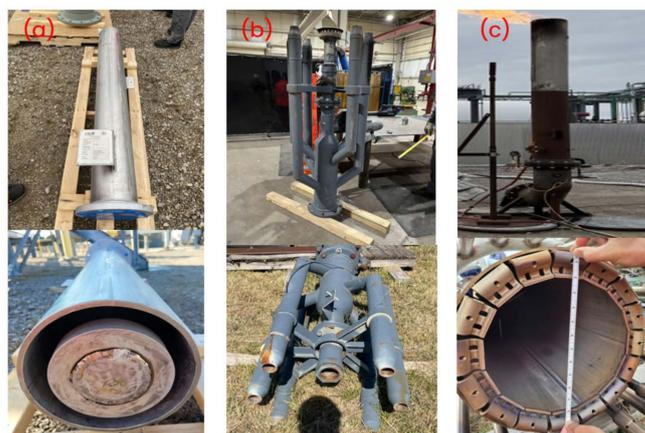
**Figure 1.** Three flare tips used for the experiment: (a) sonic—with restricted orifice shown; (b) pressure-assisted multi-arm ‘hydra’ flare tip, and (c) single-pipe non-assisted ‘utility’ flare tip.
