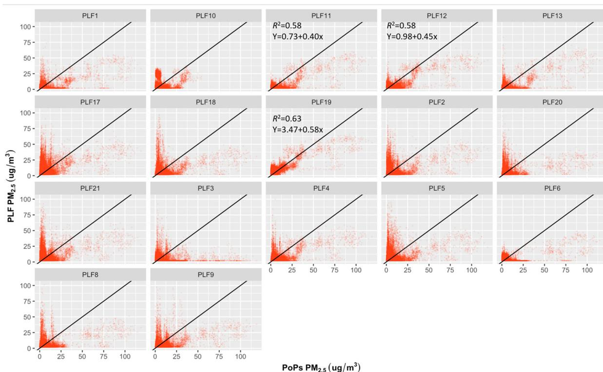
Figure 2. Regression plots for PLFs and POPS reference device for the 1 min PM<sub>2.5</sub> concentrations carried out over a three-week period at the indoor monitoring location. X-axis represents POPS reference instrument; Y-axis represents PLFs tools; ----: Black line represents the 1:1 line. For those associations between the measured PM<sub>2.5</sub> concentrations from PLFs and POPS with an R<sup>2</sup> > 0.5, the equation for linear regression is included.
