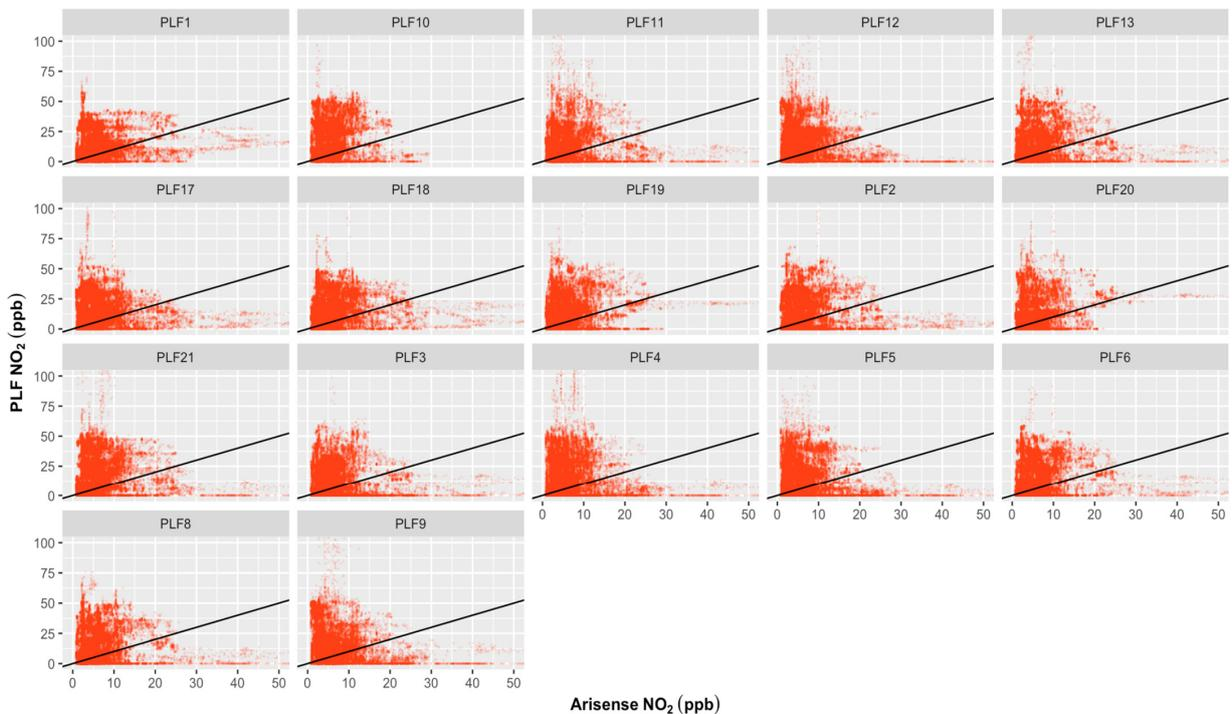
**Figure 4.** Regression plots for PLFs and ARISense reference device for the 1 min NO<sub>2</sub> concentrations carried out over a month at the indoor monitoring location. X-axis represents ARISense reference instrument; Y-axis represent PLFs tools; ---: Black line represents the 1:1 line. No linear associations between the measured NO<sub>2</sub> concentrations from PLFs and ARISense were observed. The density plot for this figure can be seen in Figure S6.
