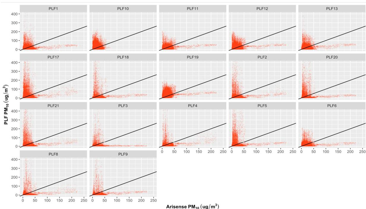
**Figure 3.** Regression plots for PLFs and ARISense reference device for the 1 min PM<sub>10</sub> concentrations carried out over a three-week period at the indoor monitoring location. X-axis represents ARISense reference instrument; Y-axis represents PLFs tools; ---: Black line represents the 1:1 line. No linear associations between the measured PM<sub>10</sub> concentrations from PLFs and ARISense were observed. The density plot for this figure can be seen in Figure S5.
