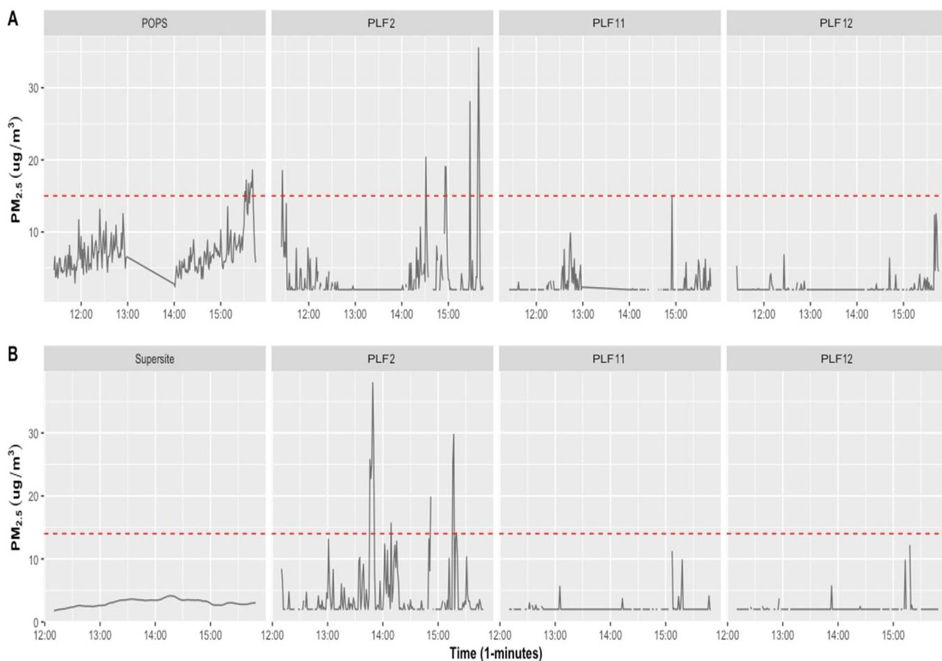
**Figure 5.** Time series of POPS and Supersite monitors (reference) and three PLF tools for PM<sub>2.5</sub>, 1 min concentrations carried out for over three hours at the (A) roadside and (B) Manchester Air Quality Supersite. To provide a reference point, the red dashed line represents the WHO limited value (15  $\mu\text{g}/\text{m}^3$  for 24 h mean PM<sub>2.5</sub>).
