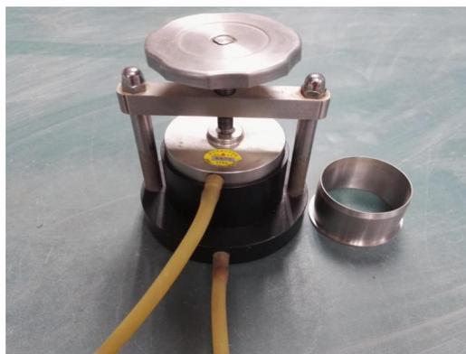
**Figure 3.** TST-55 Permeameter (Nanjing Zhongzhiyan Measurement and Control Technology Co., Ltd., Nanjing, China).
