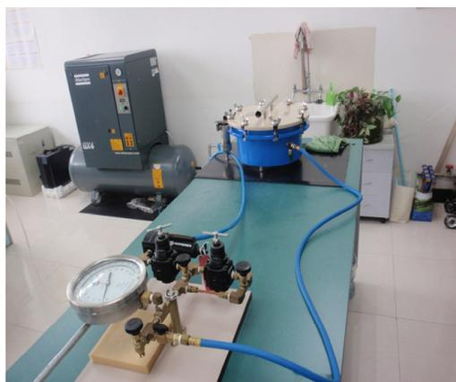
**Figure 4.** Pressure plate extractor.
