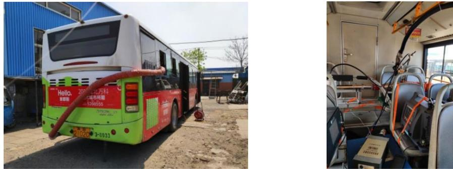
Figure 1. PEMS test vehicle on actual bus road.
