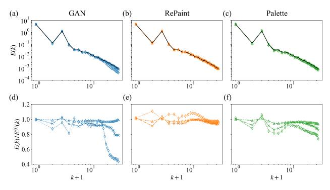
**Figure 12.** Energy spectra of the original velocity magnitude (solid black line) and the reconstructions obtained from (**a**) GAN, (**b**) RePaint, and (**c**) Palette for a square gap of sizes  $l/l_0 = 24/64$  (triangle), 40/64 (cross), and 62/64 (diamond). The corresponding  $E(k)/E^{(t)}(k)$  is shown in (**d**–**f**), where E(k) and  $E^{(t)}(k)$  are the spectra of the reconstructed fields and the ground truth, respectively.
