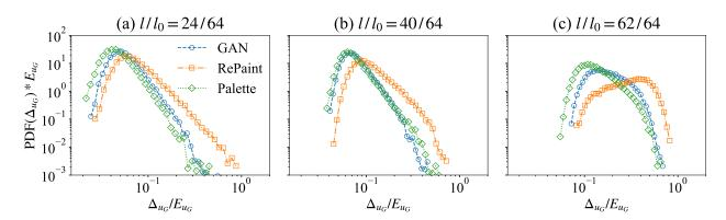
**Figure 7.** The PDFs of the spatially averaged  $L_2$  error for a single flow configuration obtained from GAN, RePaint, and Palette models. The gap size changes from (**a**)  $l/l_0 = 24/64$ , to (**b**) 40/64 and (**c**) 62/64.
