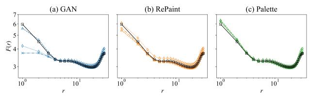
**Figure 13.** The flatness of the original field (solid black line) and the reconstructions obtained from (a) GAN, (b) RePaint, and (c) Palette for a square gap of sizes  $l/l_0 = 24/64$  (triangle), 40/64 (cross), and 62/64 (diamond).
