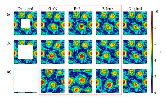
**Figure 8.** Examples of reconstruction of an instantaneous field (velocity magnitude) for a square gap of size (**a**)  $l/l_0 = 24/64$ , (**b**)  $l/l_0 = 40/64$  and (**c**)  $l/l_0 = 62/64$ . The damaged fields are shown in the first column, while the second to fourth columns, circled by a red rectangle, show the reconstructed fields obtained from GAN, RePaint, and Palette. The ground truth is shown in the fifth column.
