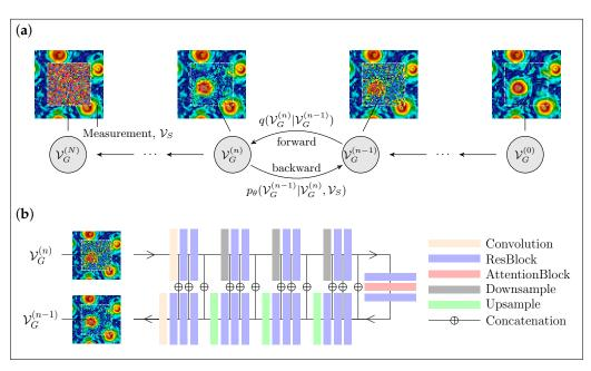
**Figure 4.** Schematic of the DM Palette protocol. (a) In the backward process (from left to right), we start from pure noise in the gap,  $\mathcal{V}_{G}^{(N)}$ , combined with the measurements in the frame,  $\mathcal{V}_{S}$ , to progressively denoise the missing information using the U-Net architecture described in (b). (b) A sketch of the U-Net integrating the measurement,  $\mathcal{V}_{S}$ , and the noisy data within the gap,  $\mathcal{V}_{G}^{(n)}$ , for a backward step.
