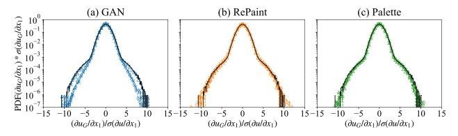
**Figure 10.** The PDFs of the gradient of the reconstructed velocity magnitude in the missing region obtained from (**a**) GAN, (**b**) RePaint, and (**c**) Palette, for a square gap of variable size  $l/l_0 = 24/64$  (triangle), 40/64 (cross), and 62/64 (diamond). The PDF of the true data over the whole region is plotted for reference (solid black line) and  $\sigma(\partial u/\partial x_1)$  is the standard deviation of the original data over the full domain.
