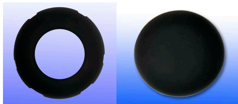
Figure 5. UV suppression: surface blackening of the deflection plate and the electrostatic analyzer.
