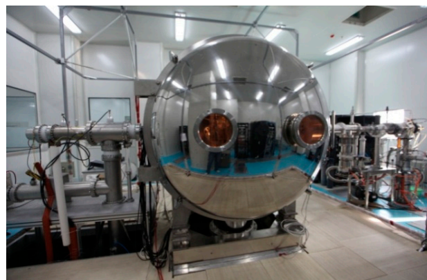
Figure 13. Low-energy particle and surface charge-discharge vacuum test system.
