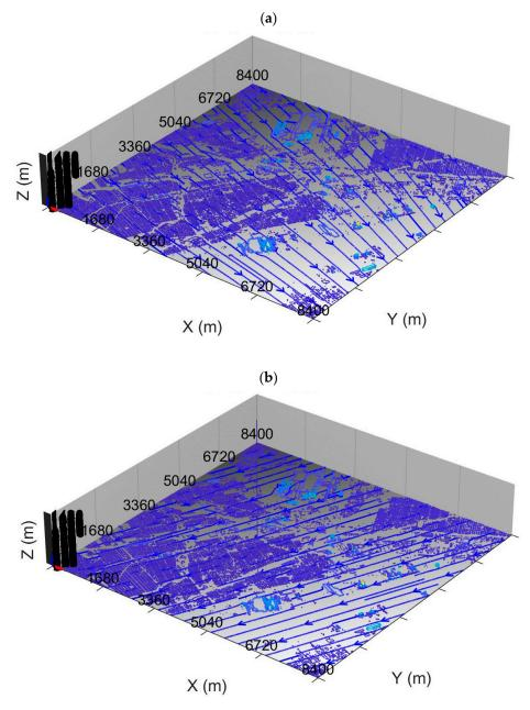
**Figure 1.** Wind streamlines (dark blue arrows) at 1 m AGL generated by the QUIC model for the Dearborn Loop area during (a) 22 May 2021, 13:13–14:13 LST and (b) 30 May 2021, 10:00–11:00 LST. Light blue colors indicate taller structures.
