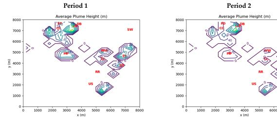
**Figure 2.** Cell-averaged plume release heights inferred from point source stack data for Period 1 (**left**) and Period 2 (**right**). See Table 3 for interpretation of red markers.
