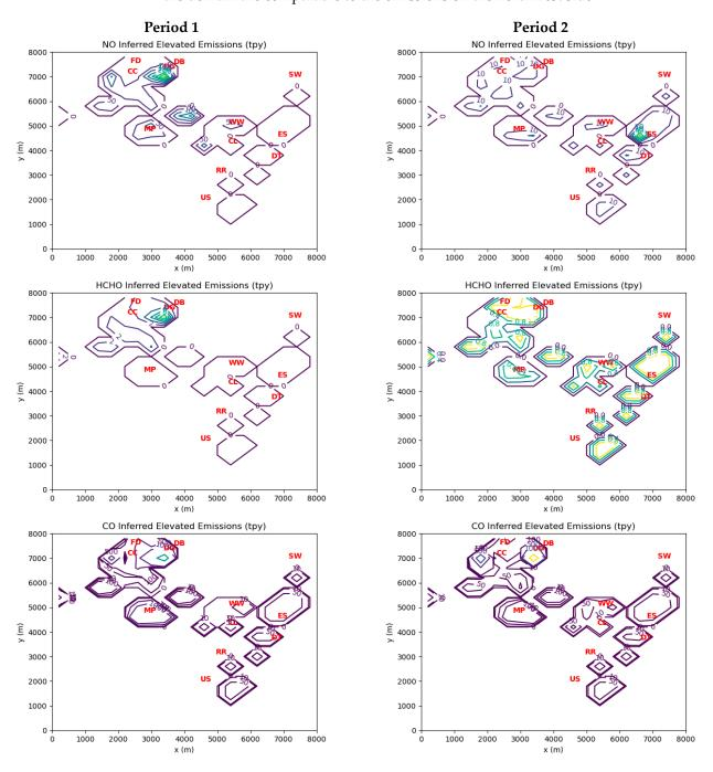
**Figure 4.** Inverse model-inferred emissions of NO, HCHO, and CO in US tons per year (tpy) for elevated sources during Periods 1 and 2. Note that contours for CO are for 10, 50, 100, 500, 1000, and 5000 tpy. See Table 3 for interpretation of red markers.
