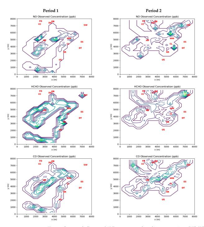
**Figure 3.** Contours of cell-averaged AML measurements for ambient concentrations of NO, HCHO, and CO during Period 1 and Period 2. See Table 3 for interpretation of red markers.
