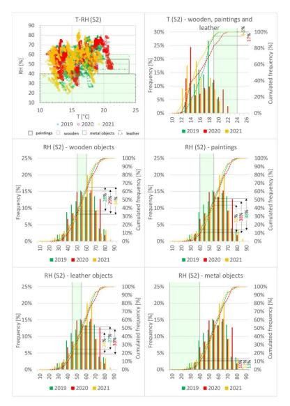
**Figure A1.** Scatterplot and frequency distribution comparison of indoor climate data (datalogger S2) from March to May 2019, 2020 and 2021 with respect to the conservation range (the green area) proposed by UNI10829 for different materials.
