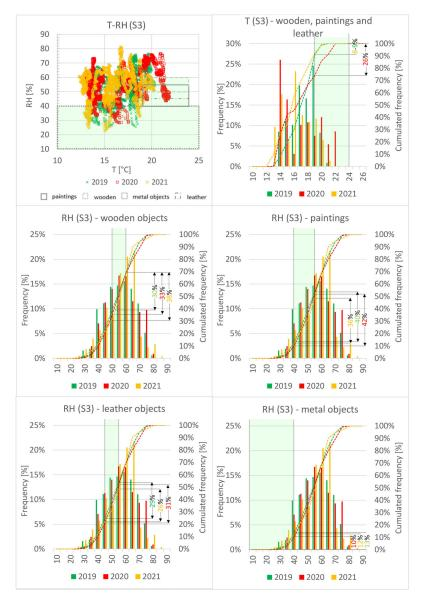
**Figure 12.** Scatterplot and frequency distribution comparison of indoor climate data (datalogger S3) from March to May 2019, 2020 and 2021 with respect to the conservation range (the green area) proposed by UNI10829 for different materials.
