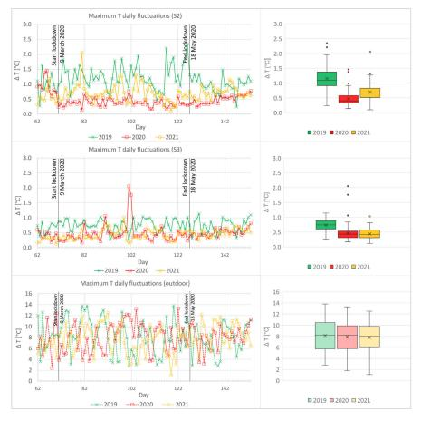
**Figure 10.** Maximum daily T fluctuation in the area close to the doors (S2), close to the organs (S3) and outdoors.
