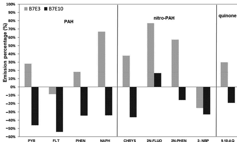
**Figure 6.** Percentage variation of individual emission of PAH, nitro-PAH, and quinones when comparing B7E3 and B7E10 with B7 for PM<sub>2.5</sub>.
