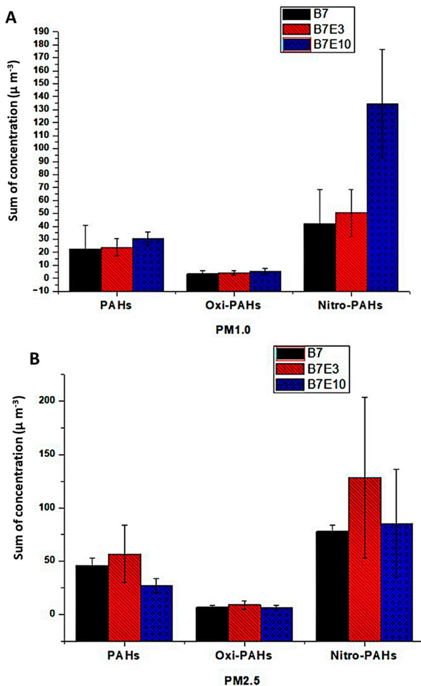
**Figure 4.** The total concentration of PAHs, quinones, and nitro-PAHs found in the particulate matter from B7, B7E3, and B7E10 blends. (A) PM<sub>1.0</sub> and (B) PM<sub>2.5</sub>.
