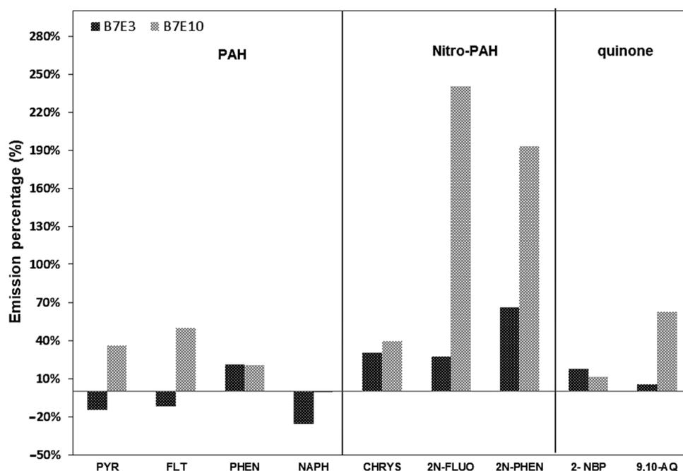
**Figure 5.** Percentage variation of individual emission of PAH, nitro-PAH, and quinones when comparing B7E3 and B7E10 with B7 for PM<sub>1.0</sub>.
