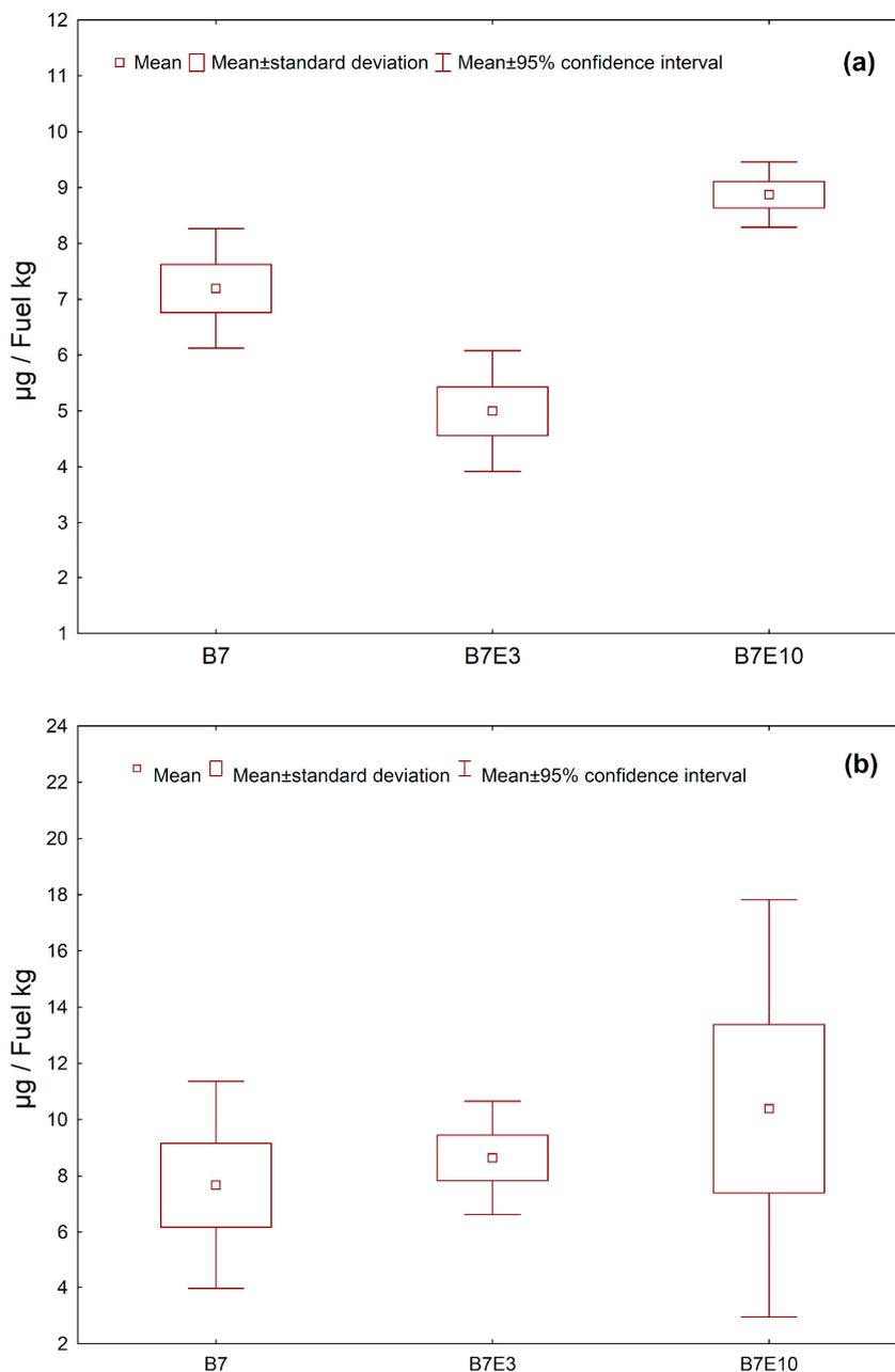
Figure 3. (a)  $PM_{1.0}$  emission factor for B7, B7E3 and B7E10 fuel blends; (b)  $PM_{2.5}$  emission factor for B7, B7E3 and B7E10 fuel blends.
