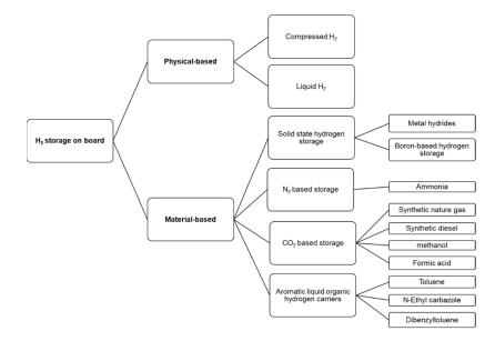
Figure 2. Potential onboard hydrogen storage technology.
