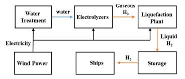
Figure 3. Offshore liquefied hydrogen production and ship refueling plant [145].
