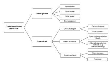
Figure 6. Production methods of green power, green hydrogen, green ammonia, and green methanol.
