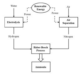
Figure 4. Green ammonia production process using green hydrogen + HB process.
