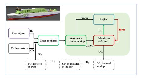
Figure 5. HyMethShip project diagram.
