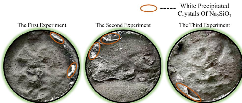
**Figure 8.** The water retention test for inorganic salt for 3# coal dust was repeated for three times at a concentration of 1 wt%, which was the best performing Na<sub>2</sub>SiO<sub>3</sub> solution for all precipitated white crystals.
