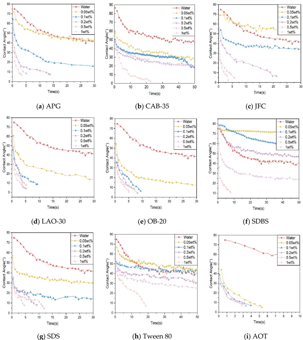
**Figure 6.** Contact angle of 3# coal dust with different surfactants at different mass fractions.
