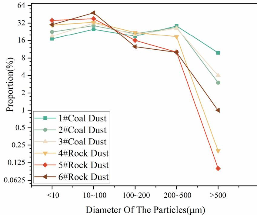
Figure 2. Particle size distribution of blast pile dust.
