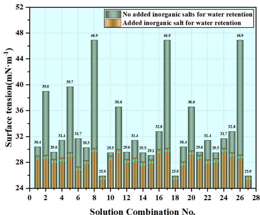
Figure 9. Changes in surface tension before and after addition of inorganic salts to surfactants.
