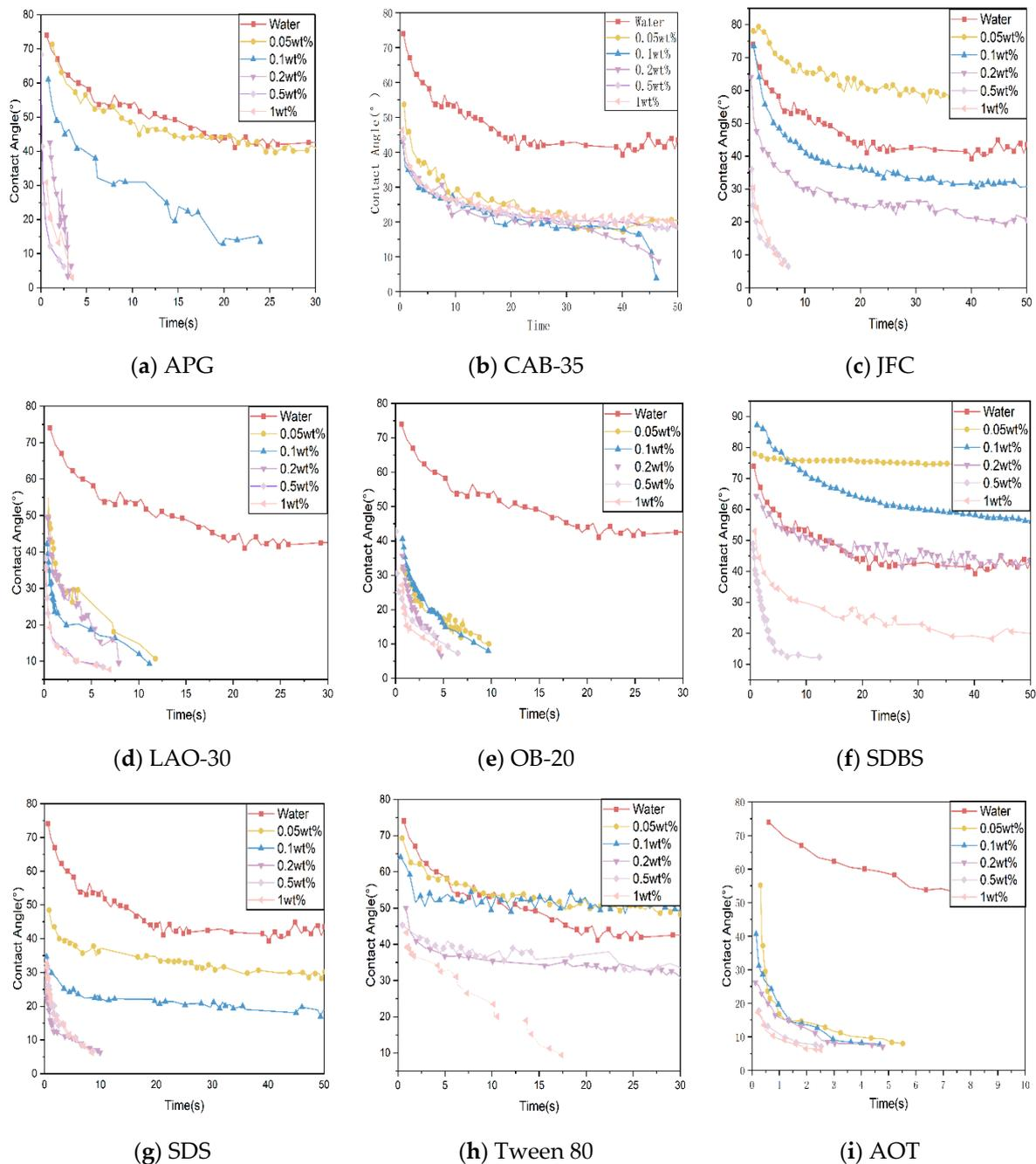
Figure 4. Contact angle of 1# coal dust with different surfactants at different mass fractions.
