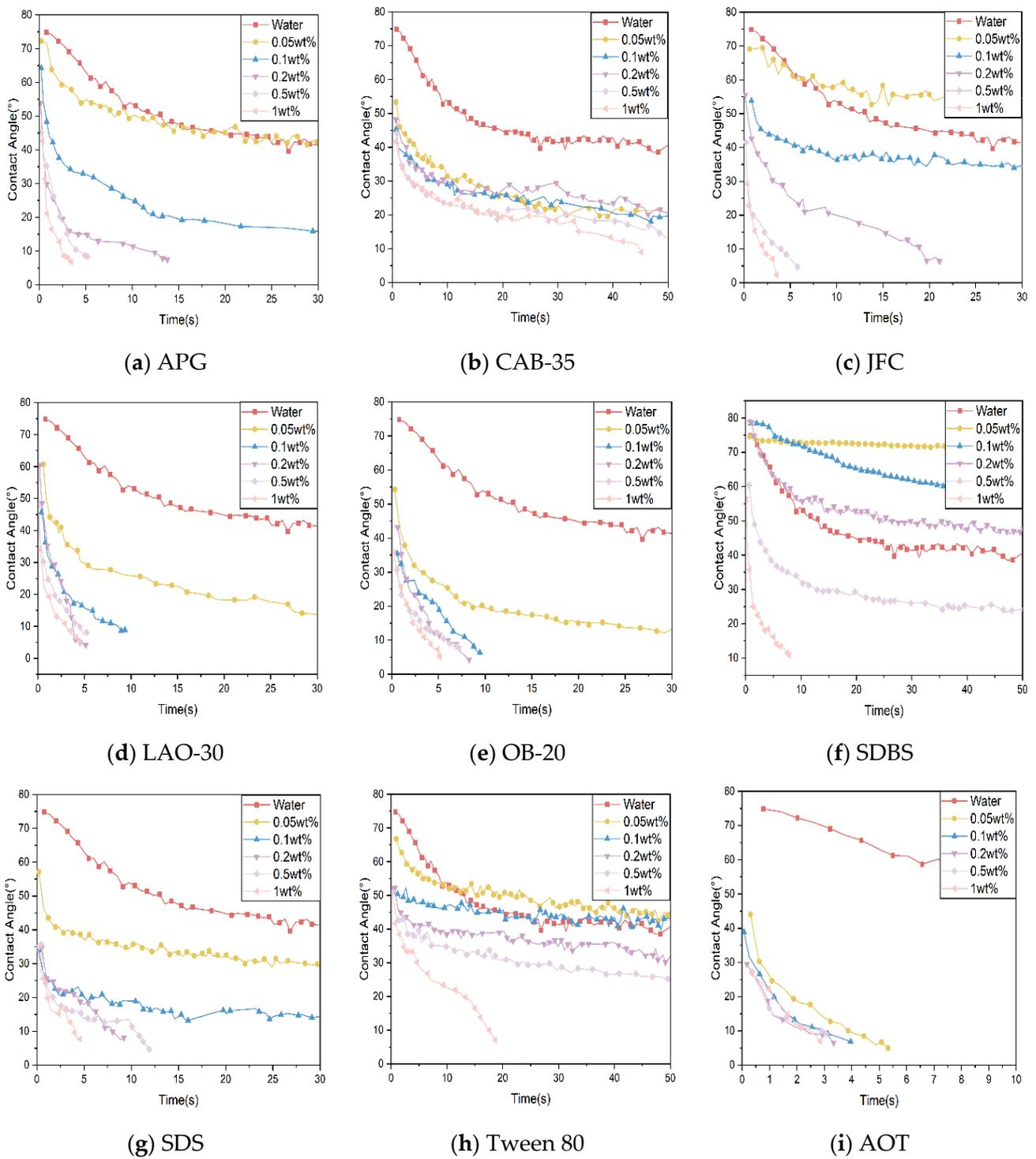
Figure 5. Contact angle of 2# coal dust with different surfactants at different mass fractions.
