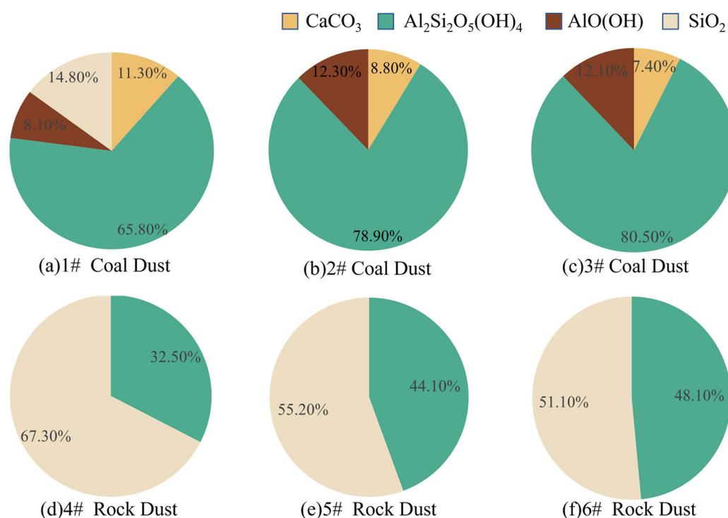
**Figure 3.** XRD analysis results of dust. (Subplots a–c show the XRD results of the three coal dust samples, and subplots d–f show the XRD results of the three rock dust samples).
