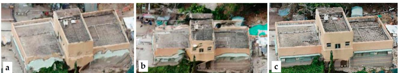
**Figure 3.** Reconstruction result of using (a) vertical photos, (b) oblique photos and (c) integrated vertical and oblique photos.
