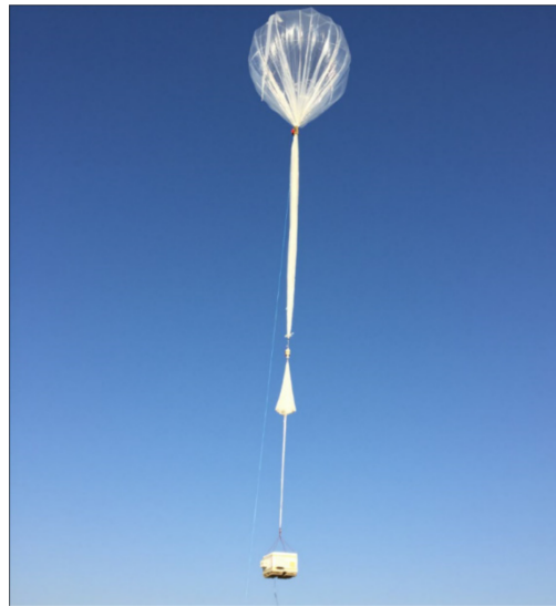
Figure 1. The radiosonde balloon equipped with the radiation detector in this study.
