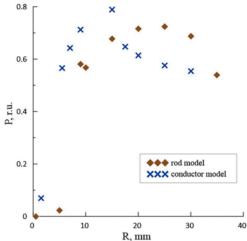
**Figure 5.** Probability of transition of a pulse streamer corona flash into an upward leader as a function of the radius of the rod electrode (radius of the tubular electrode).
