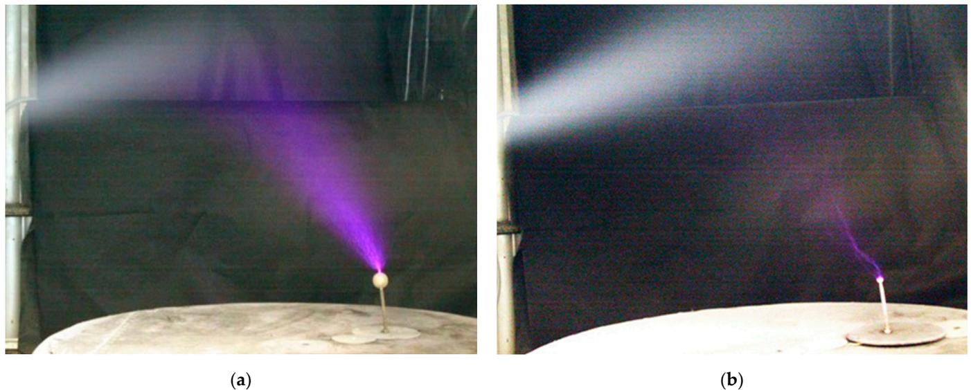
**Figure 2.** Pulse streamer corona flash (a) without upward leader transition and (b) transitioning into an upward leader.
