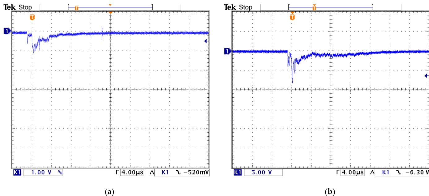
**Figure 3.** Oscillogram of the streamer corona current flowing through (a) the stem without transition into the upward leader (shunt 1.39 Ohm, 1 V/div, 4 μs/div) and (b) the stem with transition into the upward leader (shunt 1.39 Ohm, 5 V/div, 4 μs/div).
