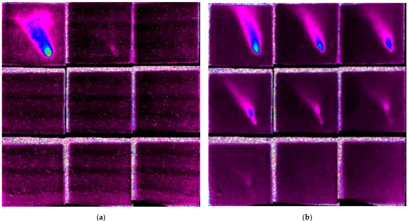
**Figure 4.** Streamer corona flash (a) without upward leader transition (frame duration  $3.5 \mu\text{s}$ , pause between frames  $0.1 \mu\text{s}$ , frame size  $0.75 \times 0.75 \text{ m}$ ) and (b) with upward leader transition (frame duration  $2.5 \mu\text{s}$ , pause between frames  $0.1 \mu\text{s}$ , frame size  $0.75 \times 0.75 \text{ m}$ ).
