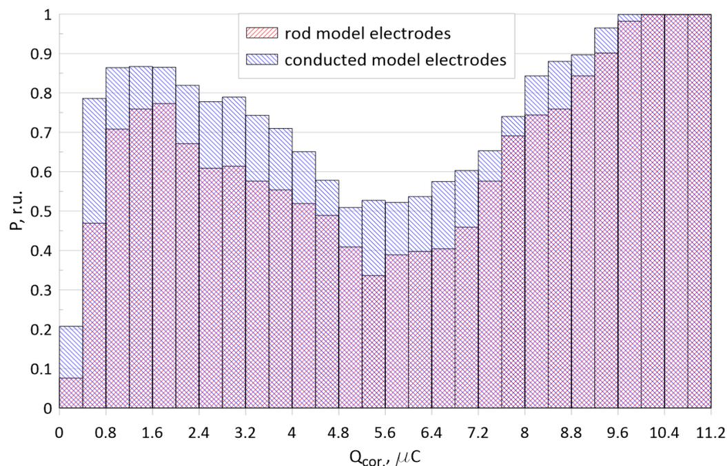
**Figure 6.** Dependence of the probability of a successful streamer–leader transition ( $P$ ) on the magnitude of the charge flowing through the base of a pulsed streamer corona flash  $Q_{cor}$  (1—rod model electrodes; 2—elongated model electrodes).
