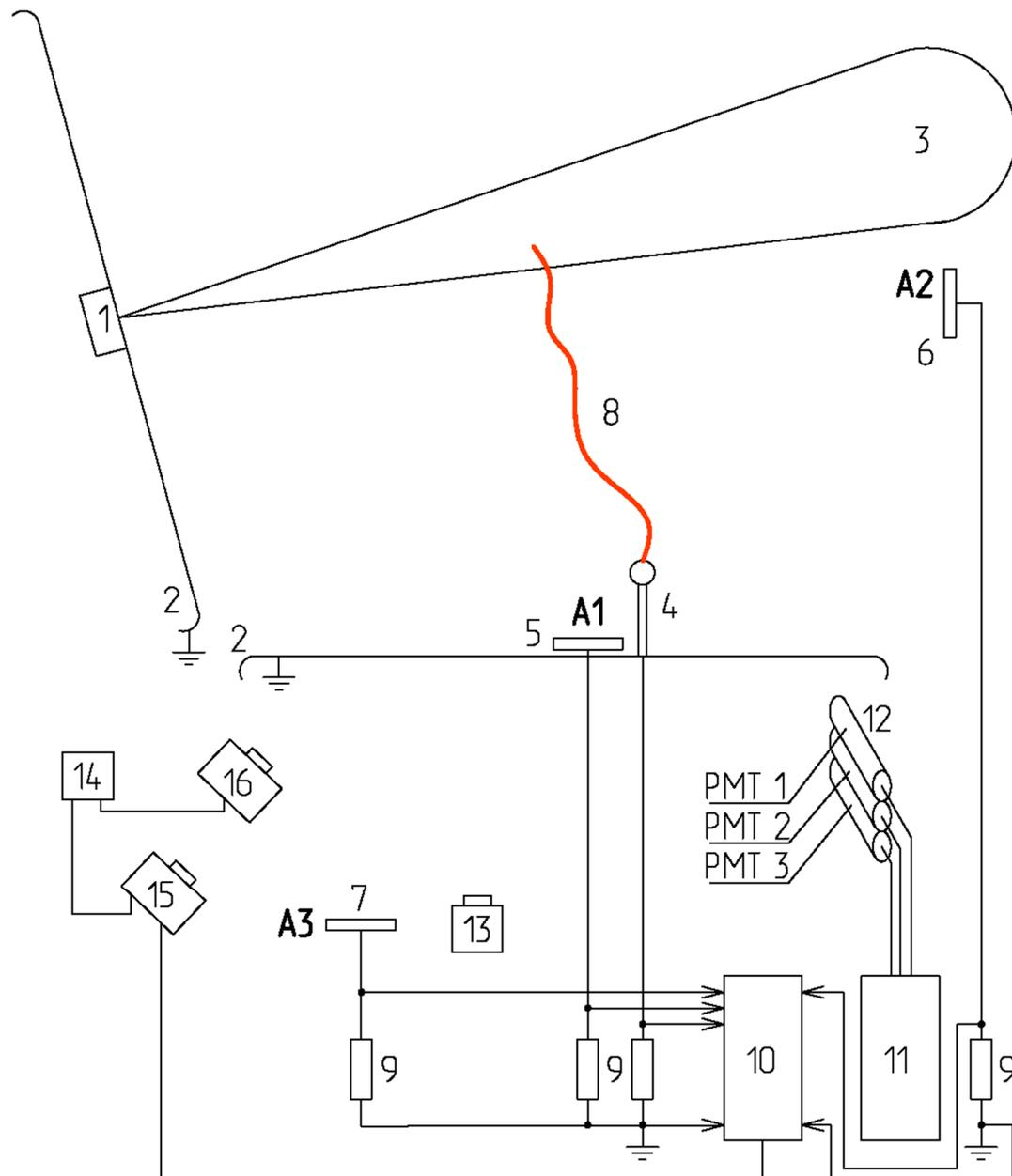
**Figure 1.** Basic scheme of the experimental measurement complex: 1—charged aerosol generator, 2—grounded electrostatic screens, 3—artificial thunderstorm cell, 4—rod or elongated model electrodes, 5–7—flat antennas, 8—spark discharges, 9—low inductive shunts, 10, 11—digital memory oscillographs, 12—a system of photoelectronic multipliers, 13—digital camera, 14—trigger generator, 15—photoelectron multiplier, 16—electron-optical camera.
